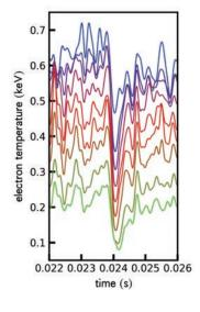
Bursty transport observed in torus plasmas. Heat is transferred to outside of plasma. This phenomenon is similar to avalanches, which are driven by self-organized criticality of turbulent plasma.
