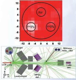
Isotope CT by using Laser-Compton Gamma-ray beam Isotope mapping by using Laser-Compton Gamma-ray beam generated in collision of electron beam and laser has been developed to apply nuclear safeguard.
