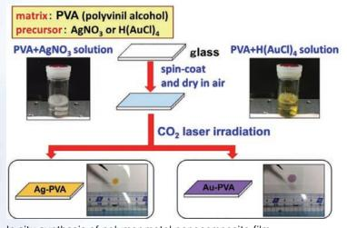
In-situ synthesis of polymer-metal nanocomposite film
