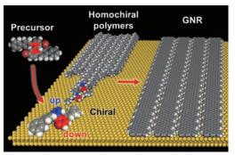
Bio-mimetic surface synthesis of graphene nanoribbons GNRs can be produced by bio-mimetic principles consisting of chiral transformation, of designed z-bar-linkage precursors, self-assembly, homochiral polymerization and dehydorogenation.
