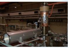
High-power microwave source "Gyrotron"
