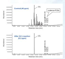
D. The result of reacting 40 mg L<sup>-1</sup> of commercial PCBs with composite type of catalytic enzyme, it degraded to 0.3 mg L<sup>-1</sup> in comparison with the control (top) within 24 hours (bottom). PCBs was analyzed by gas chromatograph quadrupolemass spectrometer.
