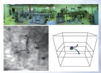
The interaction between vacancy cluster induced by ion accelerator and a dislocation: comparison between experimental study and computational study.
