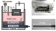
A new production method of solar-grade silicon by the electrochemical reduction of silica in molten salt
