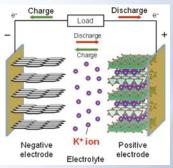
Principle of potassium-ion battery
