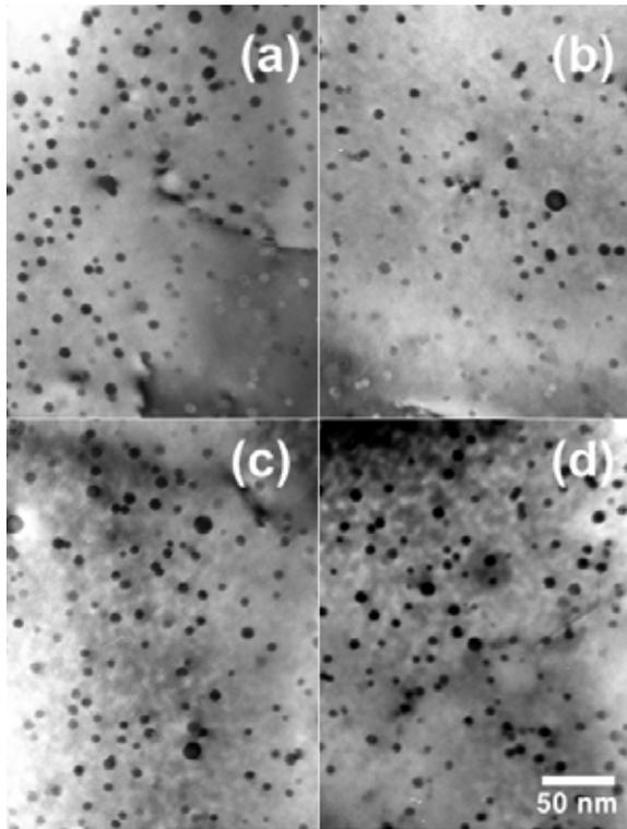
Fig. 4. Transmission electron micrographs, showing a thermally aged 22Cr (K5) ODS steel at temperature 475 °C up to (a) 5, (b) 50, (c) 505 and (d) 1000 hours, respectively, black dots=oxide particles, bright field images.
