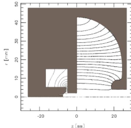
Fig. 10: Schematic cross-section of an rf gun with an rf-powered triode structure.
