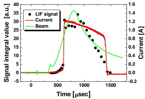
Fig. 8: Time distribution of exciter current and LIF signals by pulsed helium beam
