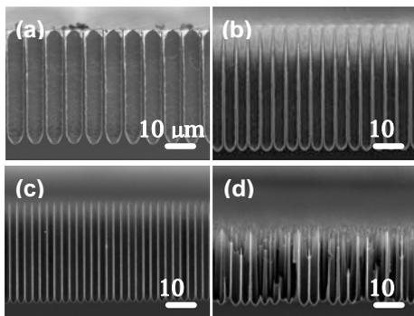
Fig. 4-1 Cross-sectional FE-SEM images of prepatterned silicon wafers after anodization in HF solution at 13 mA/cm<sup>2</sup> for 2 hours. The spacing of etch pits is (a) 8, (b) 5, (c) 3, and (d) 2 μm.
