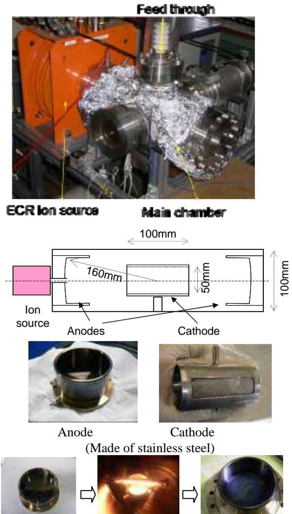
Fig. 3. New type of fusion source with Ti coated electrodes.
