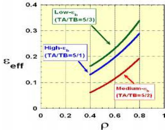
Fig.1 Calculated “effective” helical ripple  $\epsilon_{eff}$  as a function of radius for high- $\epsilon_b$ , medium- $\epsilon_b$  and low- $\epsilon_b$  configurations.
