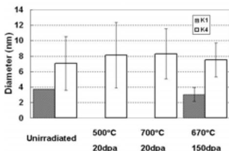
Fig. 4: Irradiation effects for diameter of dispersed oxides of both (Y, Ti) complex oxides in K1 alloy and (Y, Al) complex oxides in K4 alloy.
