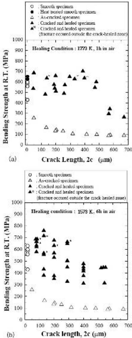
**Fig. 2 Effect of pre-crack length on the bending strength of crack healed specimen at room temperature: (a) crack healed at 1773 K, 1 h, (b) crack healed at 1573 K, 6 h.**
