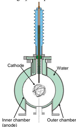
at a large negative potential. Ions are accelerated to the center as they gain energy from the applied electric fields and the spherical focusing of ions results in a high ion density inside the grid. The use of a highly transparent cathode grid minimizes the ion loss to the grid and allows the significant recirculation of energetic ions.
