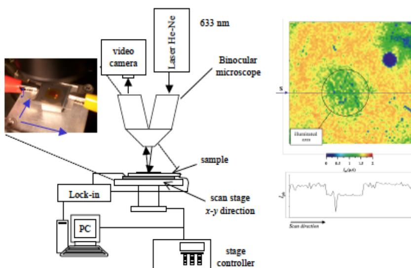
**Fig. 4** Instrument (left) of Laser Beam Induced Current (LBIC) and photocurrent image (right) of DSC after illumination of fluorescence light through the circular mask for 3 week.
