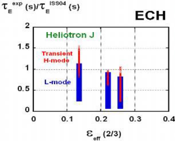
**Fig.2** Confinement enhancement factor,  $H_{ISS04}$ , with regard to the ISS04 scaling as a function of  $\epsilon_{eff}$  at  $r/a=2/3$  for ECH plasmas with the bumpiness modified configurations.
