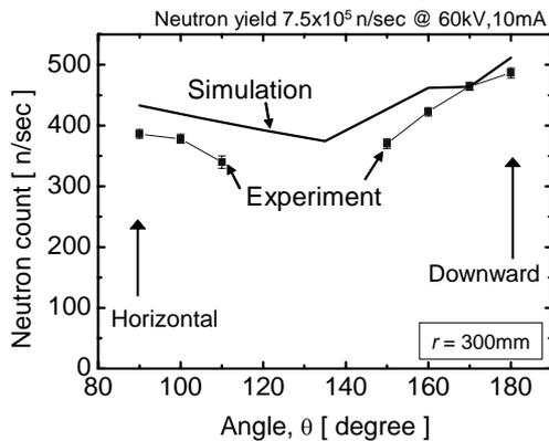
Fig. 3. Experimental and numerical results of neutron count rates obtained by  $^3\text{He}$  proportional counter
