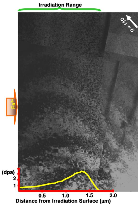
Fig.8: TEM bright field image of ion-irradiated area of Fe-1.5Mn model alloy.
