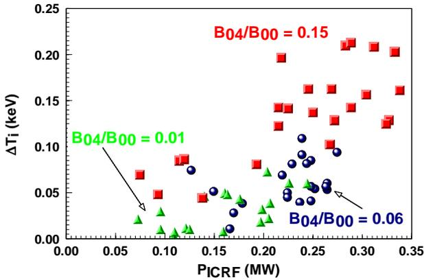
Fig. 3 Increase of the bulk ion temperature as a function of the injected ICRF power for three bumpy cases.
