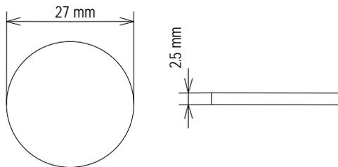
Fig. 10 Schematic drawing of the YBCO test piece.
