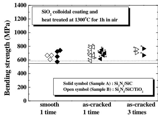
**Fig. 4 Effect of crack-healing according to coating time.**
