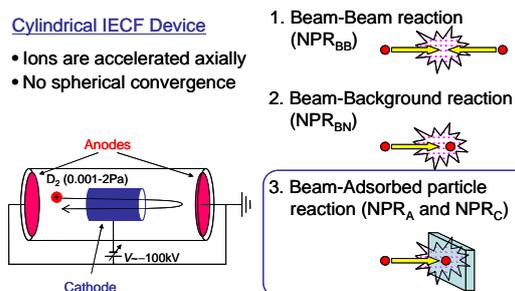
Fig.1 Collision processes in IECF device.
