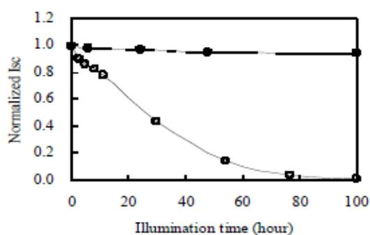
**Fig. 3** Durability of ITO/PEDOT:PSS/P3HT:PCBM/TiO<sub>2</sub>/Al under an atmospheric illumination at light intensity of 100 mW/cm<sup>2</sup>, AM 1.5.
