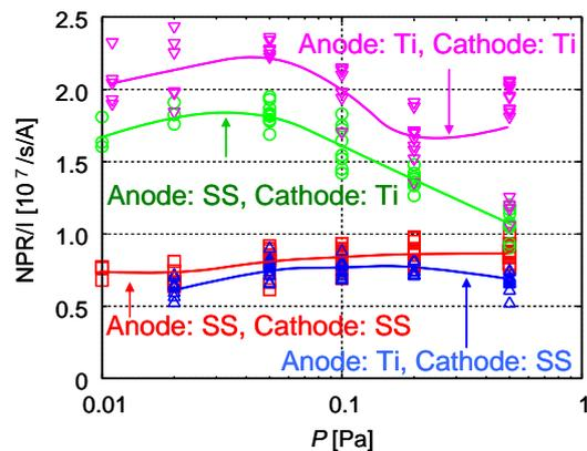
Fig.4 Experiments on neutron production rates by various combination of surface reactions.
