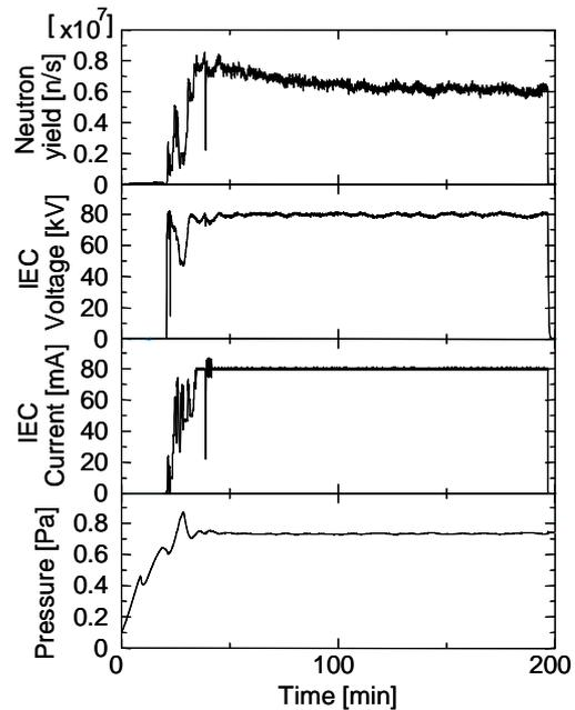
Fig. 2. A typical run of the NEG-based IECF device
