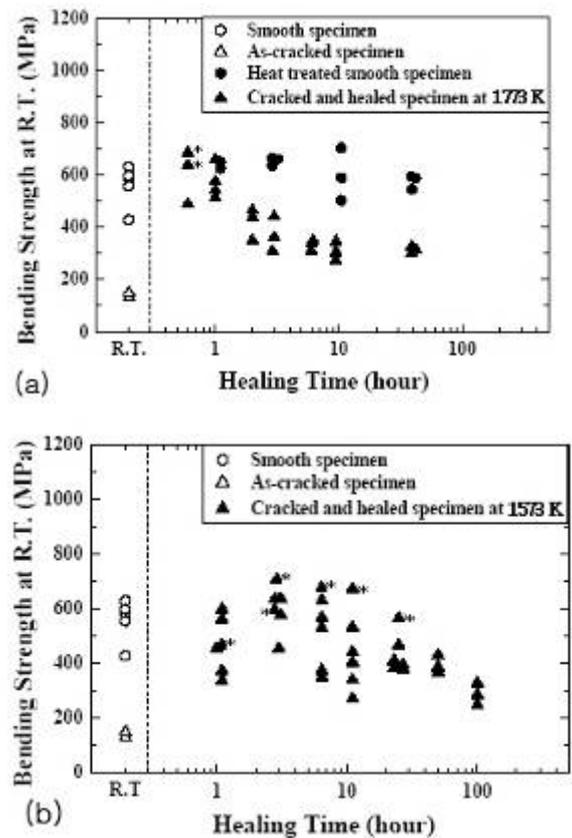
**Fig. 1 Relationship between crack-healing time and bending strength at room temperature. Data marked with (\*) indicate that fracture occurred outside the crack-healed zone: (a) crack healed at 1773 K, (b) crack healed at 1573 K.**
