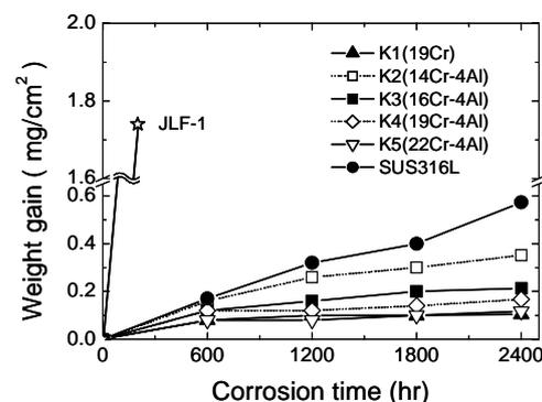
Fig. 1: The weight gains of the high-Cr ODS ferritic steels as well as those of a 9Cr martensitic steel (JLF1) and an austenitic stainless steel (SUS316L) in a super critical pressurized water (783 K, 25 MPa).
