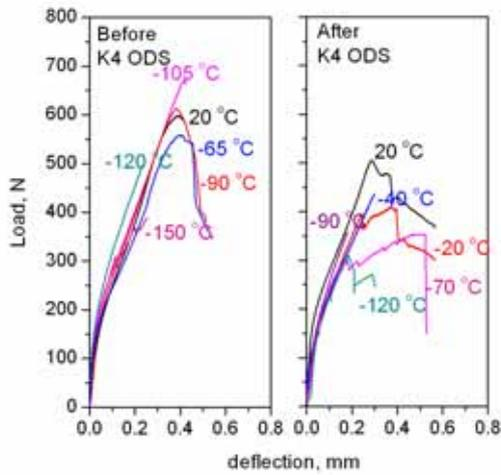
Fig. 1. SP load-deflection curves of 19Cr ODS (K4) steel before and after thermal aging treatment at 437 °C for 322 hours.
