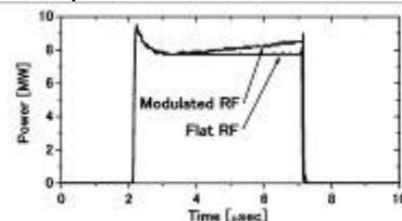
Fig. 5 Input RF power fed to the RF gun
