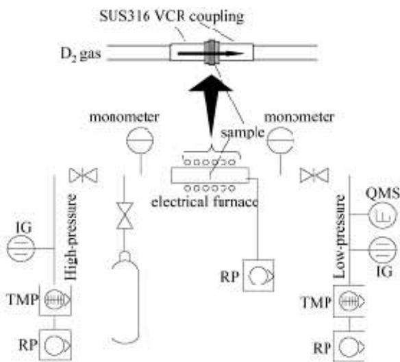
Fig.8 A schematic diagram of the experimental setup for hydrogen permeation through blanket materials.
