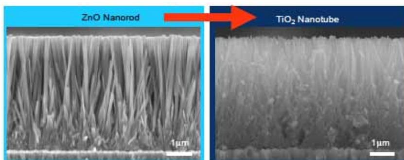
**Fig. 7** TiO<sub>2</sub> nanotube array from ZnO template.
