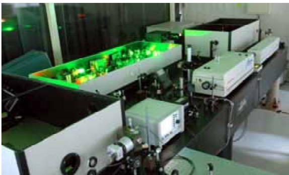
**Fig.1.** High-intensity fs Ti:sapphire CPA laser system.
