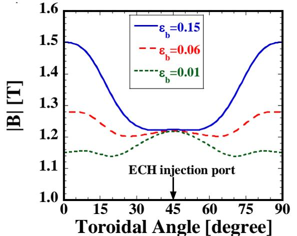
FIG. 3. Magnetic field strength along magnetic axis. The arrow denotes the EC wave injection position.
