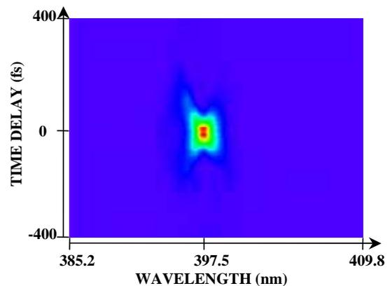
**Fig.2.** Example of the FROG image for the 100-fs, 800-nm laser pulse.
