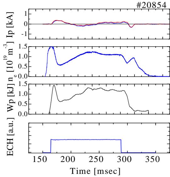
FIG. 4. Time evolution of ECH plasma with net free current.
