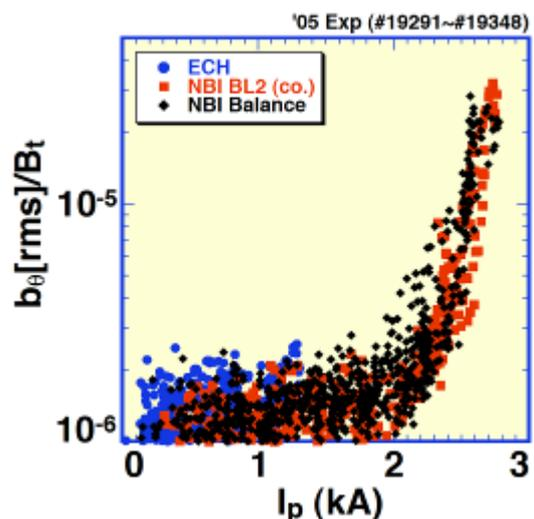
*Fig.1* Statistic analysis of the amplitude of MHD mode against the plasma current.
