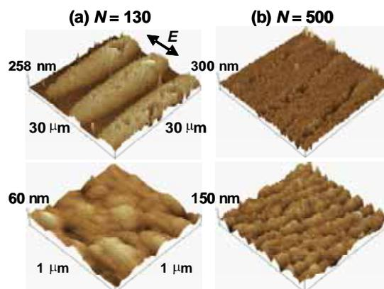
**Fig.6.** SPM images of DLC surfaces at 130 and 500 shots of fs laser pulses. The upper images are  $30 \times 30$   $\mu m^2$ , and the lower are  $1 \times 1$   $\mu m^2$ .
