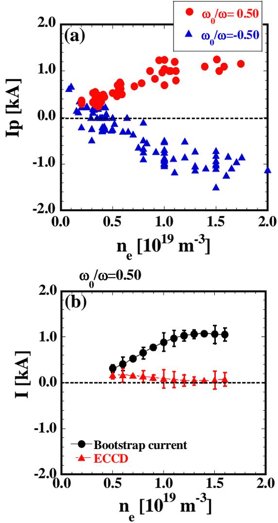
FIG. 1. Density dependence of non-inductive current at medium configuration, (a) measured total toroidal current at  $\omega_0/\omega = +0.50$  and  $\omega_0/\omega = -0.50$ , (b) estimated bootstrap and EC currents.
