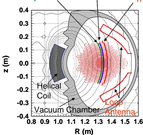
Fig. 1 Two ICRF antennas in the corner section of Heliotron J.
