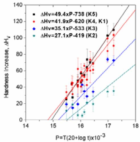
Fig. 3. (a) Vickers micro-hardness (Hv) as a function of the aging time in each ODS steel, thermally aged at 475 °C and (b) increase in Vickers micro-hardness ( $\Delta H_v$ ) as a function of the aging parameter  $P$ ,  $P=T(20+\log t)\times 10^{-3}$ , where  $T$  is the temperature and  $t$  is the aging time.
