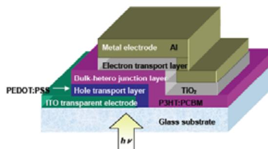
**Fig. 1** Structure of organic thin film solar cell.
