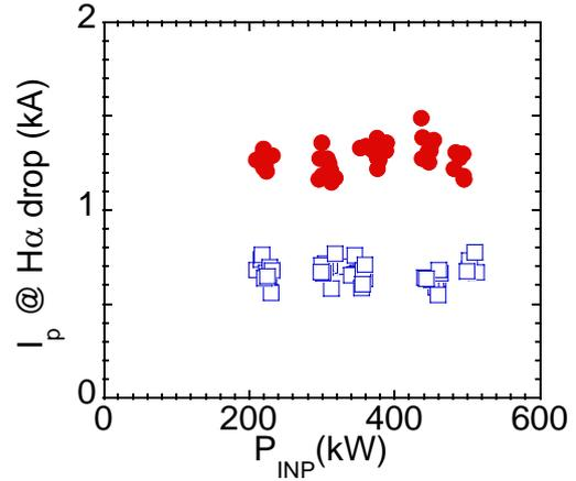
FIG. 7. Plasma toroidal current at the drop of  $H\alpha$  line intensity as a function of NB power.
