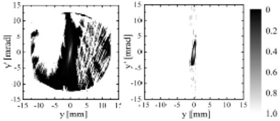
(a) Tomographic method (b) Single slit method
