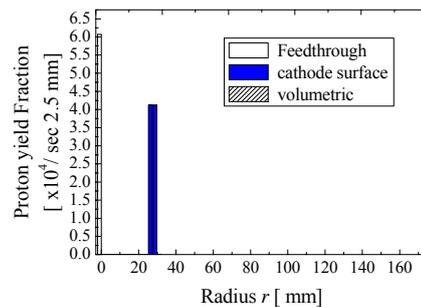
Fig. 6: Reconstruction of  $D\text{-}^3\text{He}$  proton distribution ( the bias voltage at -51 kV, grid current at 28.5 mA, and  $P_{3\text{He}}/P_{\text{total}}=0.75$ )
