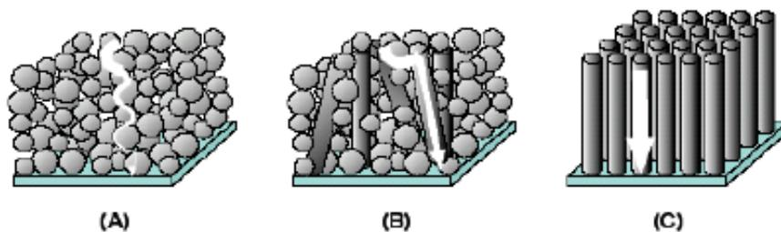
**Fig. 5** “Electron expressway concept” by using 1D or 2D nanosized metal oxides as electron transport layer or electrode for organic solar cell; (A) Conventional nanosized grains, (B) 1D nanowires with grains, (C) 2D arrays of nanorods..
