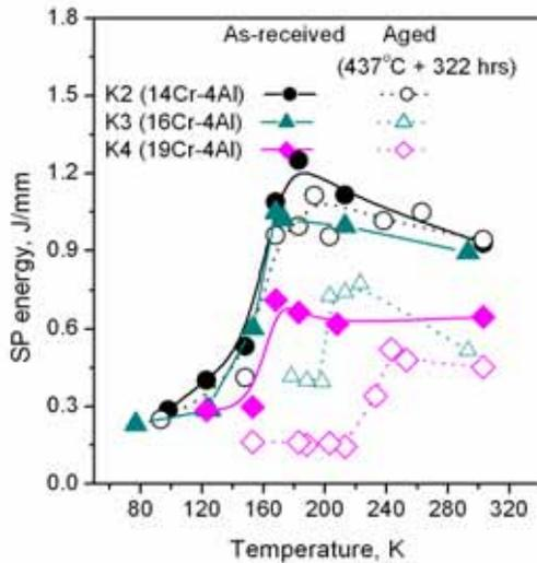
Fig. 2. Effects of thermal aging treatment on the specific SP energy of the ODS steels as a function of test temperature, for samples thermally aged at 437 for 322 hours.
