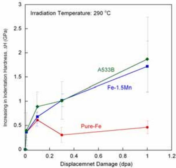
Fig.7: Dose dependence of irradiation hardening of Pure Fe, Fe-1.5Mn and A533B after Fe-ion irradiation estimated by nano-indentation hardness tests.
