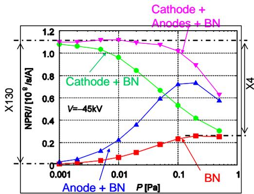
Fig.2 Calculated neutron production rates by various combination of surface reactions.
