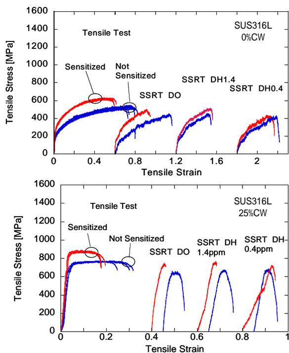
Fig. 5: Stress-strain curves of the SUS316L with and without cold-working and sensitization obtained from SSRT in dissolved oxygen and dissolved hydrogen condition.
