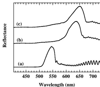
Fig. 7-1 Reflectance spectra of rugate filters before (a) and after exposure to saturated vapors of methanol (b) and (c) ethanol for 15 min.
