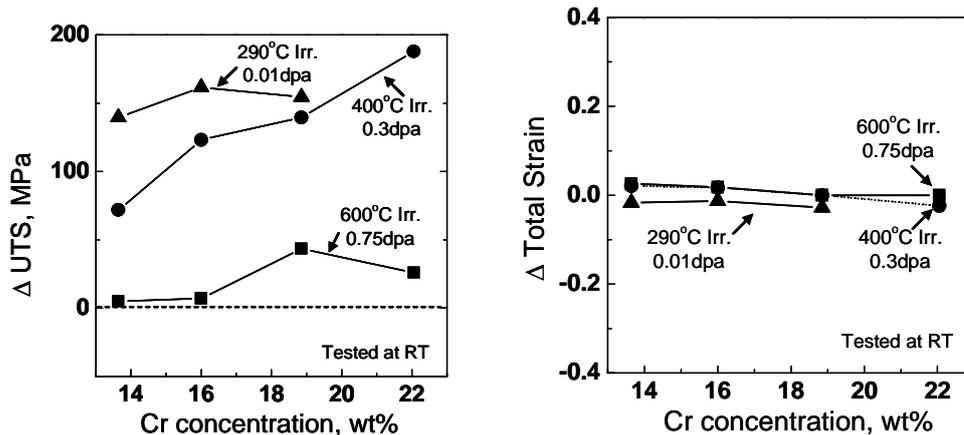
Fig. 2: Changes of a) ultimate tensile strength and b) total strain with various Cr concentrations after irradiation. Tensile test were done at room temperature at a strain rate of  $6.7 \times 10^{-4} \text{ s}^{-1}$ .
