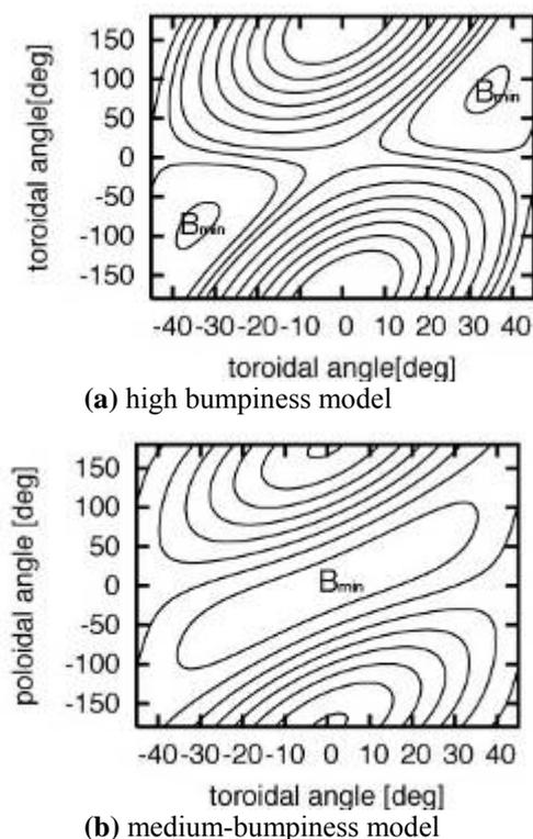
**Fig.7** The mod- $B$  contours of high and medium bumpiness models of Heliotron J. Figure shows that toroidal localization of mod- $B_{\min}$  is realized in high bumpiness model
