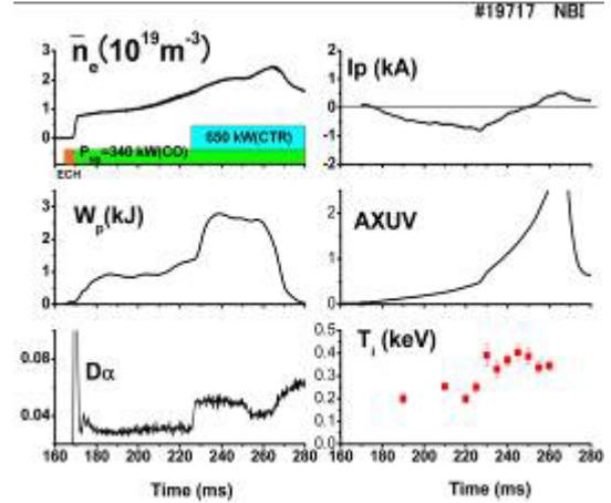
**Fig.3** Time evolutions of plasma parameters in the stage-injection of NBI (CO and CO+CTR) in the medium- $\epsilon_b$  configuration.
