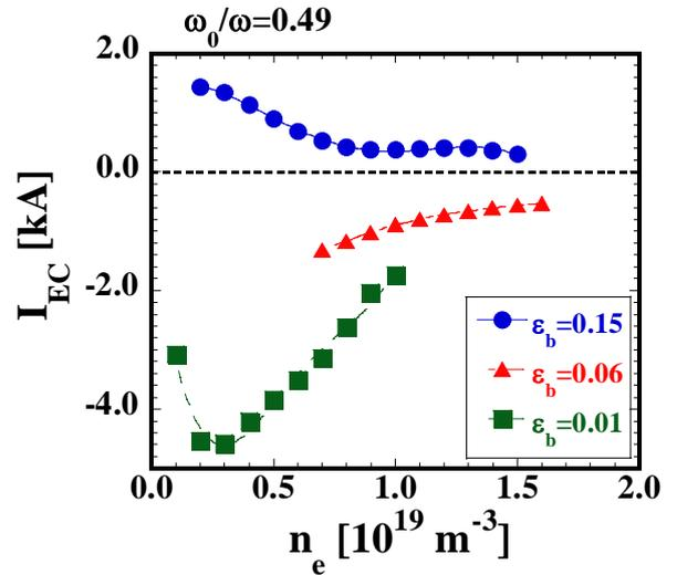
FIG. 2.  $n_e$  dependence of ECCD at  $\omega_0/\omega = 0.49$  at several field configurations.
