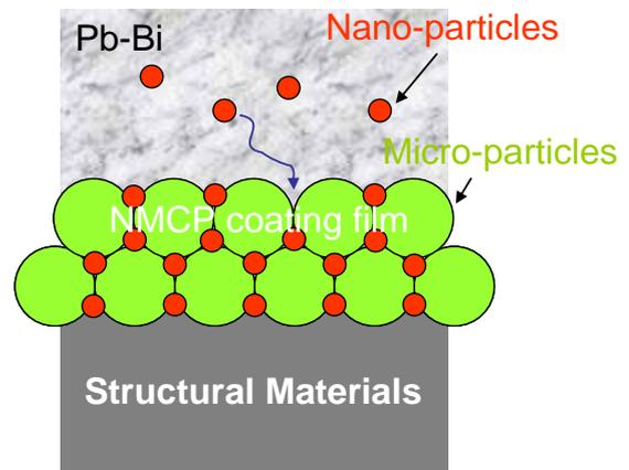
Fig.9: Schematic of the NMCP coating against LBE corrosion.
