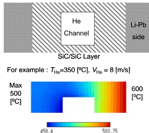
Fig.6 Temperature distribution in the SiC cooling panel. The right side faces 900 degree LiPb while the left is maintained below 550 degree.
