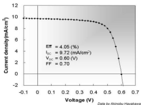
**Fig. 2** I-V curve and cell efficiencies of ITO/PEDOT:PSS/P3HT:PCBM/TiO<sub>2</sub>/Al.
