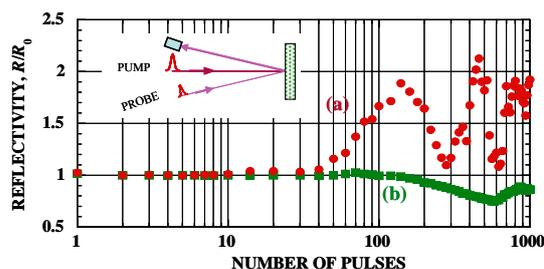
**Fig.5.** Example of the reflectivity of DLC film measured as a function of shot number with the pump and probe pulses.
