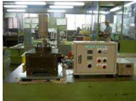
Fig.10: Rotating specimen corrosion testing system.
