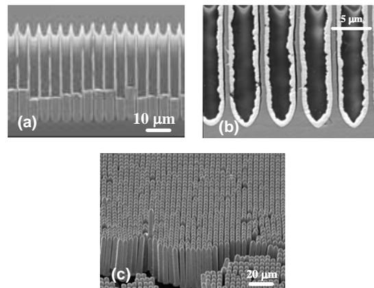
Fig. 5-1 Metal deposition into macropores. (a) copper deposition in the dark, (b) nickel deposition under illumination, and (c) after dissolution of the silicon template.
