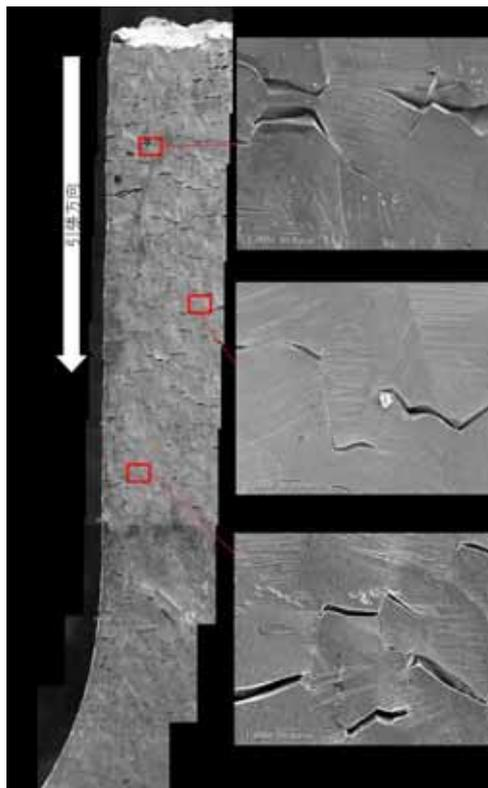
Fig. 6: SEM image of the SSRT specimen surface tested in the DH condition for the 0%CW SUS316L.
