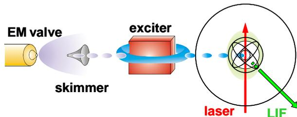
Fig. 7: Schematics of a pulsed injector of a supersonic metastable helium beam as a beam probe for the Laser-Induced Fluorescence method
