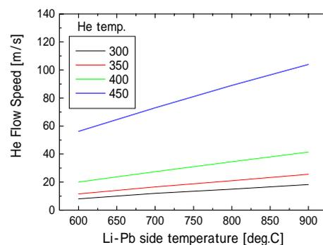
Fig.7 He flow speed and possible blanket temperature.
