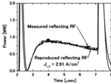
Fig. 8 Measured and reproduced reflected RF waveform from the RF gun
