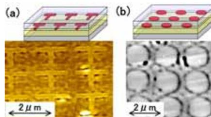
Fig. 3. (a) AFM images of photoresist TDMR-AR87 developed using a T-shaped array photomask. (b) AFM images of photoresist TDMR-AR87 using a circle-shaped array photomask.
