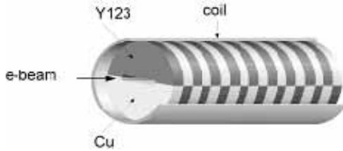
Fig. 9. Conceptual drawing of the high  $T_C$  SC undulator.
