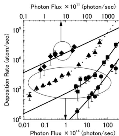
Fig.2. The optical power (photon-flux:  $I$ ) dependency of the rate  $R$  of Zn deposition.
