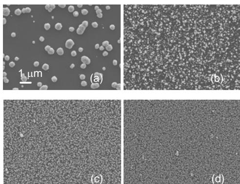
Fig. 6-1. SEM images of Cu-deposited p-type silicon. Electrodeposition was conducted in aqueous solution containing 4 mM  $\text{CuSO}_4$  (a) in the dark, under illumination of (b) 12.5, (c) 25, and (d) 50  $\text{mW/cm}^2$ .
