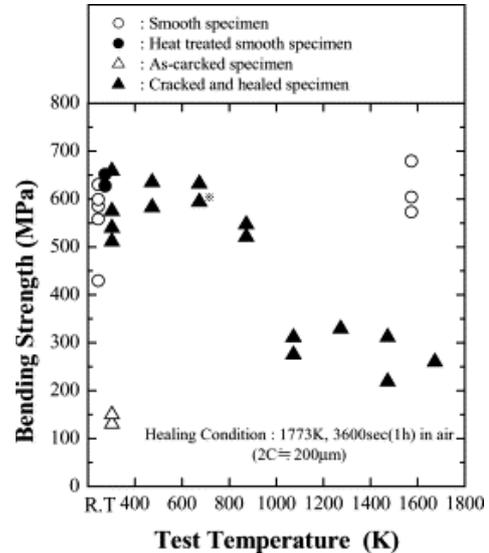
**Fig. 3 Effect of test temperature on the bending strength of crack-healed specimen.**
