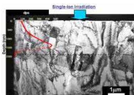
Fig. 3: Cross section of the irradiated surface of K1 ODS steel.
