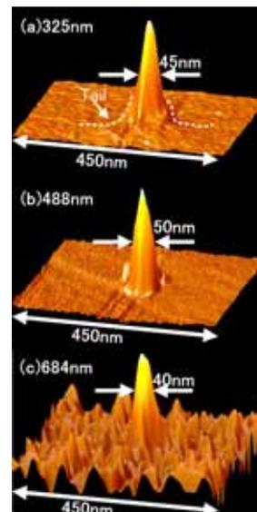
Fig. 1 . Shear-force topographical images after NFO-CVD at wavelengths of  $\lambda = 325$  (a), 488 (b), and 684 (c) nm.
