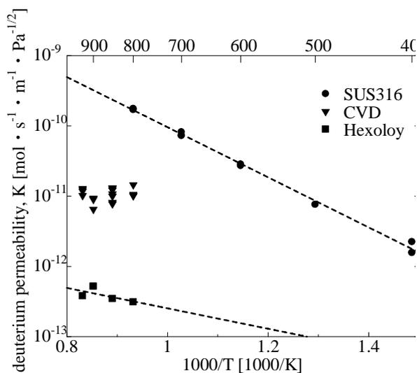
Figure 9 shows the temperature dependence of deuterium permeation in Arrhenius form. It was expected that SiC provides a very low permeability of tritium, but the present study showed the large difference between Hexoloy, (sintered alpha-SiC) and CVD beta SiC. Further measurement will continue to optimize the SiC composite material to be used.
