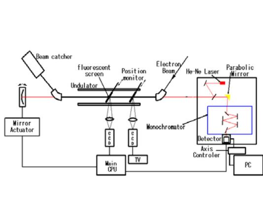
Fig. 2 Experimental setup for measurement of spontaneous radiation
