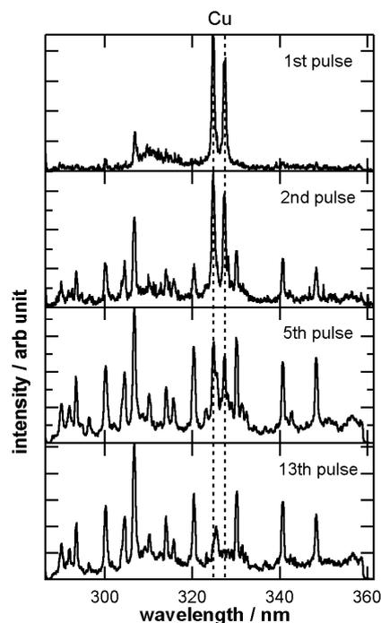
Fig. 2-1. Spectrum obtained by consecutive irradiation of the same spot on the Cu thin film electrodeposited on a Pt plate. The intensity is normalized to the highest peak in the spectrum. The spectral lines other than 324.75 and 327.40 nm are all assigned to atomic Pt.
