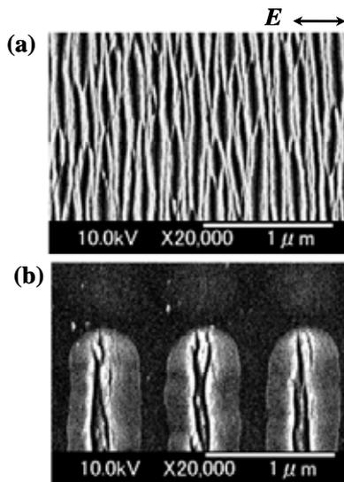
**Fig.7.** SEM images of (a) the non-patterned DLC surface irradiated with  $N = 1000$ , and (b) the patterned surface with  $N = 100$ . Both were irradiated at  $F = 80$   $\text{mJ}/\text{cm}^2$ .
