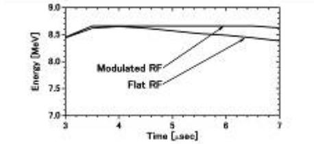
Fig. 7 Time evolution of the peak beam energy
