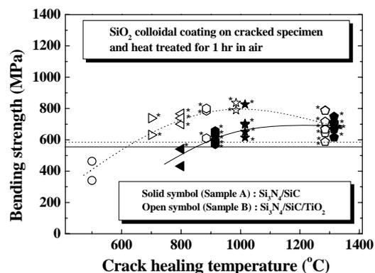
**Fig. 5 Effect of crack-healing according to heat treated temperature of as-cracked specimen with SiO<sub>2</sub> colloidal**
