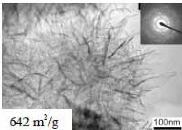
**Fig. 6** TiO<sub>2</sub> nanosheet..
