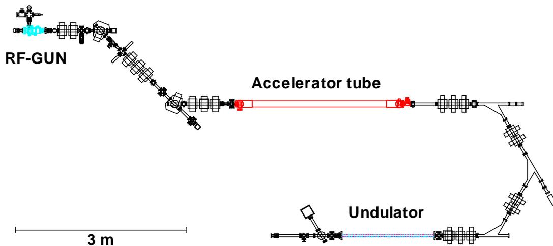
Fig. 1 Schematic drawing of the KU-FEL
