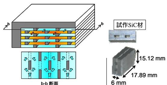
Fig.10 typical structure of the compact heat exchanger and the sample of the SiC composite cooling channel structure.
