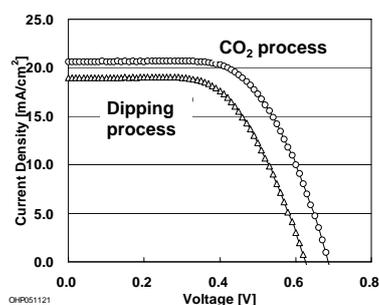
Figure 2. Photovoltaic properties for cells prepared by CO<sub>2</sub> and dipping processes
