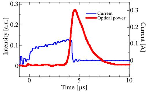
Fig. 2 Temporal evolutions of the electron beam current and the optical output
