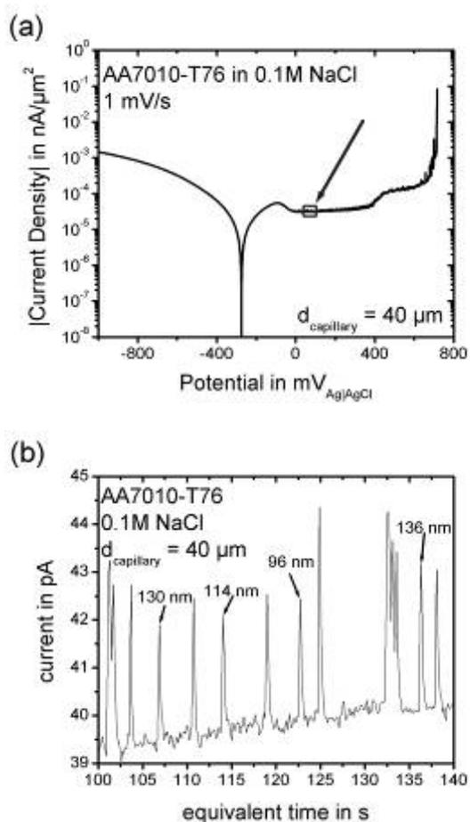
in using the microcapillary technique to study the local electrochemical behavior of specific surface sites of heterogeneous substrates, such as different intermetallic particles, the particle/matrix-interface, pure matrix, or grain boundaries. These studies can help to identify “weak sites” of the surface, or enable to understand formation of internal galvanic couples on alloy surfaces. Examples of such investigations can be found in Refs. [4-6].
