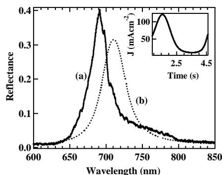
Fig. 7-1 Reflectance spectrum of a 100-cycle PSRF formed by a modified sinusoidal current density shown in the inset (a) and that simulated by assuming a sinusoidal variation of the refractive index with the depth (b).
