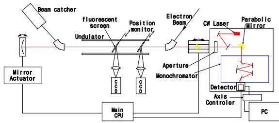
Fig. 3 Experimental setup for measurement of the FEL output
