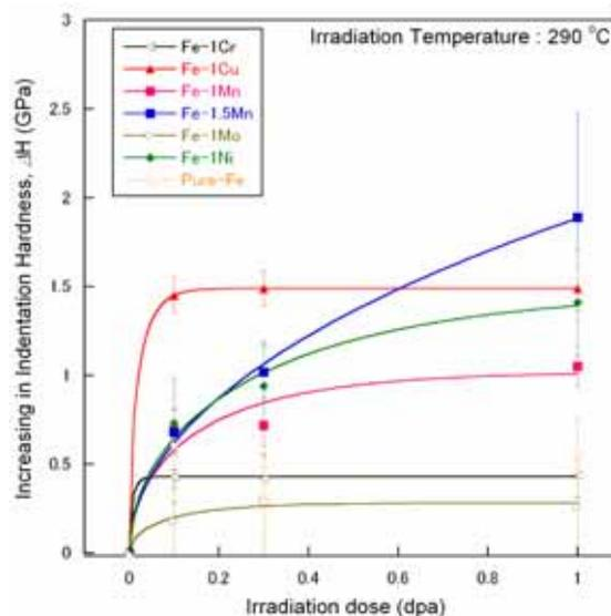
Fig. 5 Fitting curves for the dose-dependence of irradiation hardening of Pure-Fe and Fe-based binary alloys by using  $\Delta H = A[1-\exp(-B \times \text{dpa})]^{0.5}$ .
