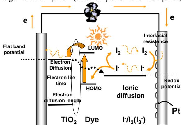
Figure 1. Working principle of DSCs
