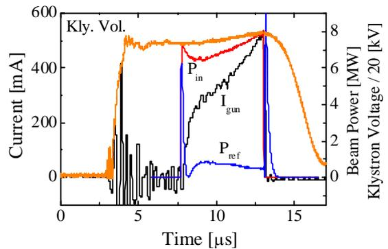
Fig. 6. Time evolution of the Klystron voltage (Kly. Vol.), the input and reflected RF power ( $P_{in}$ ,  $P_{ref}$ ), and the extracted beam current from the RF gun ( $I_{gun}$ )
