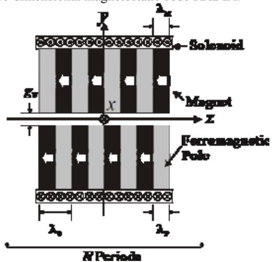
Fig. 13. Conceptual drawing of the high  $T_c$  hybrid SC undulator.
