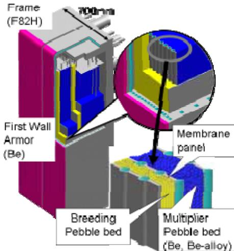
Figure 2 Concept of Solid-breeding water-cooled TBM design
