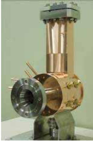
Fig. 11 Photograph of the newly manufactured photo-cathode RF gun.
