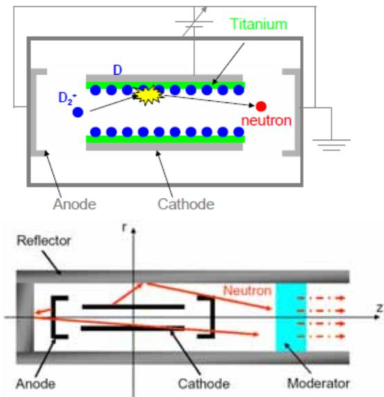
Fig.2 Models of the beam neutron source; the upper is the Ti coated discharge chamber, the lower is for the neutronics calculation.
