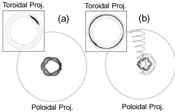
**Fig. 5. Trapped ion orbits starting in the straight section for the high bumpy case (a) and the medium bumpy case (b).**
