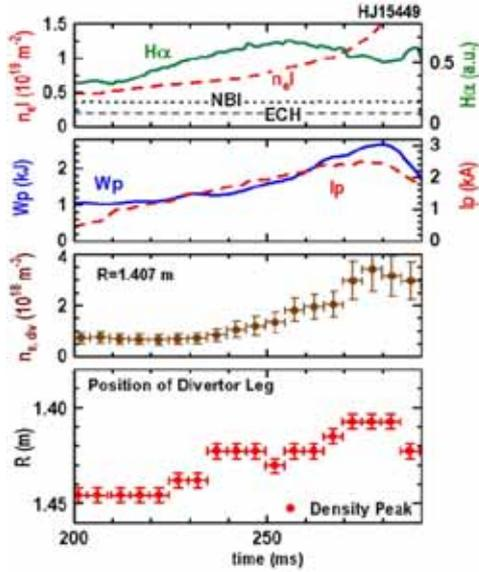
Fig. 6. Time traces of several signals for an ECH and NBI combination heating discharge in the STD configuration ( $B_0 = 1.25$  T).
