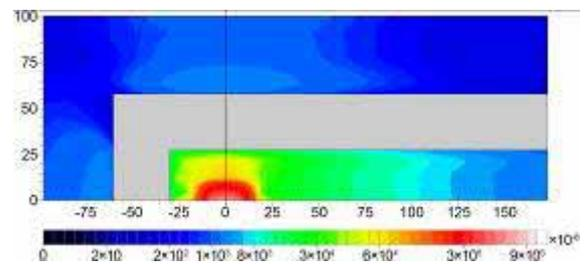
Fig. 3(b). Two dimensional neutron flux generated with the cylindrical reflector configuration..
