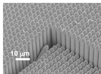
Fig. 5-1 FE-SEM image of ordered Pt micro-rods obtained by electrodeposition of Pt into macroporous Si at -0.3 V for 4 h under dark condition. The Si template was removed by chemical etching in alkaline solution.
