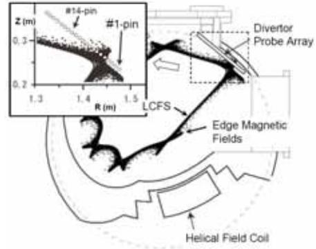
Fig. 5(a) Poincaré plot of the edge field lines at the divertor probe array section ( $\phi = 67.5^\circ$ ). The inset shows the probe-pin positions.
