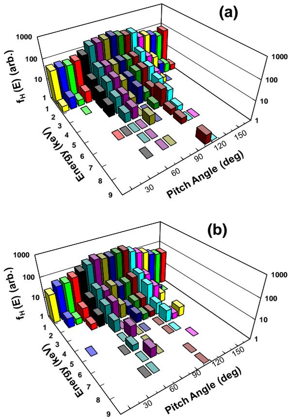
**Fig. 6. Calculated pitch angle dependence of energy spectra in the high bumpy case (a) and the medium bumpy case (b).**
