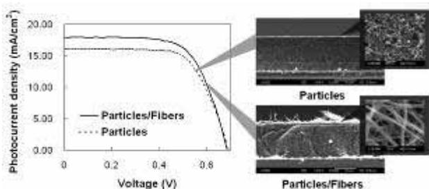
**Fig. 3** I-V curves (left) and SEM images (right) of DSCs with or without TiO<sub>2</sub> nanofibers.
