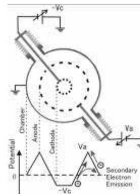
Fig. 8: Schematics of the double-grid IECF.
