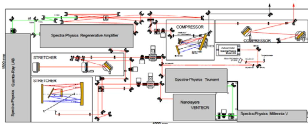
Fig.1. 10-fs Ti:sapphire CPA laser system under development.
