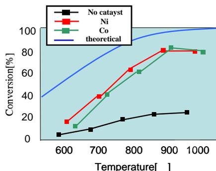
Fig.7 Hydrogen production as the results of the catalytic reaction
