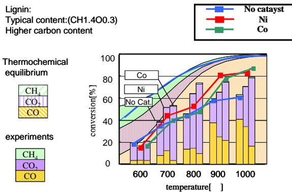
Fig.8 Gaseous products of Carbon compounds generated by the thermal decomposition of lignin followed by various catalysts
