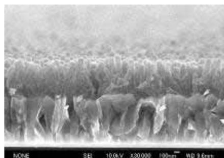
**Fig. 1** SEM image of  $\text{TiO}_2$  nanotube arrays on FTO prepared from  $\text{ZnO}$  nanorod array through template liquid phase deposition method (S.Y. *et. al.*, *Chem Lett.*, **2007**, *36*, 1508-1509).
