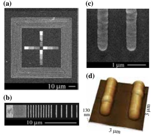
**Fig.4.** SEM images of (a) the patterned Si substrate, (b) an array of stripes in the central area, (c) the DLC-coated stripes at 800-nm period, and (d) SPM image of the same stripes as in (c).
