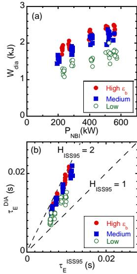
Fig. 2. (a) Stored energy obtained in high, medium and low  $\epsilon_b$  configurations as a function of NBI power and (b) comparison between  $\tau_E^{\text{DIA}}$  and  $\tau_E^{\text{ISS95}}$  in NBI sustained plasmas.
