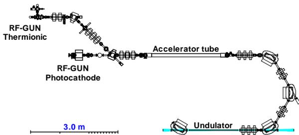
Fig. 12 Upgrade design of the KU-FEL
