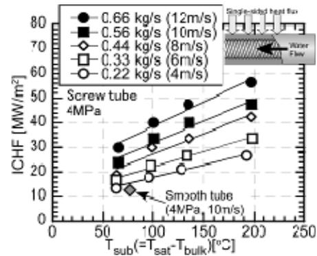
Figure 4 Effect of subcooling on ICHF of Cu screw tube
