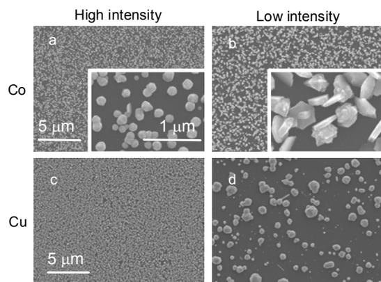
Fig. 6-1 SEM images of Co and Cu deposits on p-type Si under illumination of high and low intensities. Applied potential was  $-0.6$  V and  $-0.1$  V, respectively.
