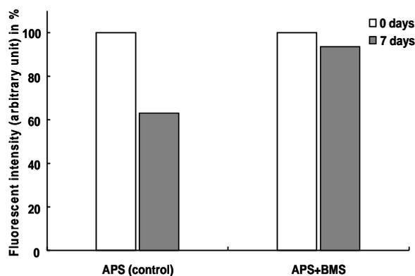
**Figure 2.** Fluorescence intensity of Cy3-labelled complementary targets hybridized with probe DNA on array surface at 0 days (white bar) and after 7 days exposure to 42°C temperature and 50% humidity (grey bar).
