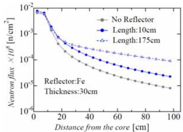
Fig.3 (a) Neutron flux along the axis with various reflectors.
