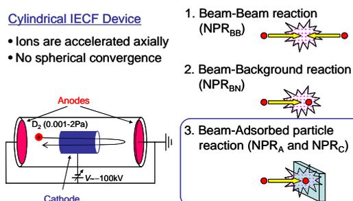
Fig.1 Collision processes in a discharge device.
