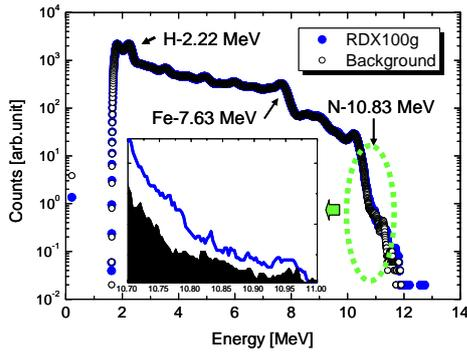
Fig. 5: BGO spectra for RDX 100g buried 15 cm deep in soil moisture of 10 wt%, and without RDX, i.e. the background.
