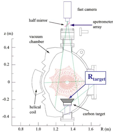
Fig. 5(b) Schematic view of the rail-limiter type carbon target and the fast-camera image monitoring system.
