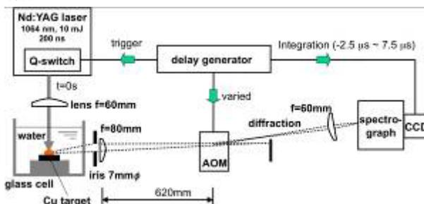
Fig. 2-1. Experimental setup for the use of AOM to gate the detection of emission spectra from the laser ablation plume produced by a solid target in water.
