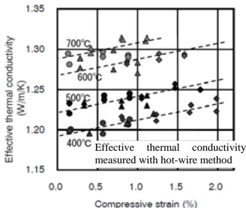
Figure 3 Effective thermal conductivity of a compressed  $Li_2TiO_3$  pebble bed.
