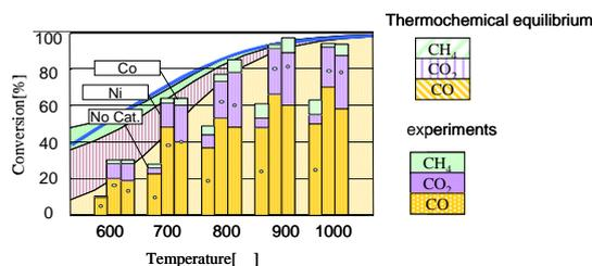
Fig.6 Gaseous products of Carbon compounds generated by the thermal decomposition of cellulose followed by various catalysts.
