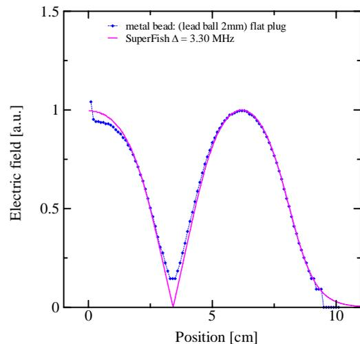
Fig. 10 Electric field distribution in the photocathode RF gun measured using microwave cavity perturbation technique.
