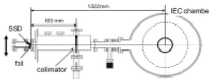
Fig. 6: Layout of the proton measurements with a movable SSD and collimator.
