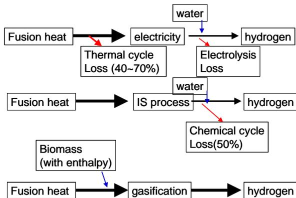
Fig. 10 comparison of fusion energy utilization with various conversion processes.
