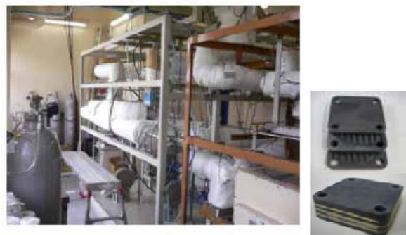
Fig.11 Test loop of the liquid LiPb, and test specimen of heat exchanger structure made with SiC composites.
