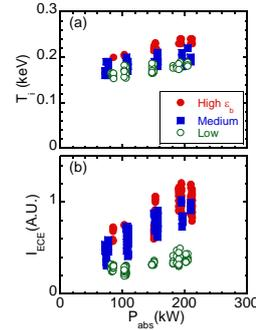
Fig. 3 (a) Bulk (deuterium) ion temperature and (b) ECE intensity as a function of  $P_{\text{abs}}$  in high, medium and low  $\epsilon_b$  configurations.
