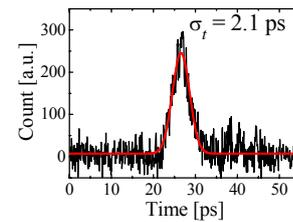
Fig. 2: Typical result of bunch length measurement by using a streak camera.
