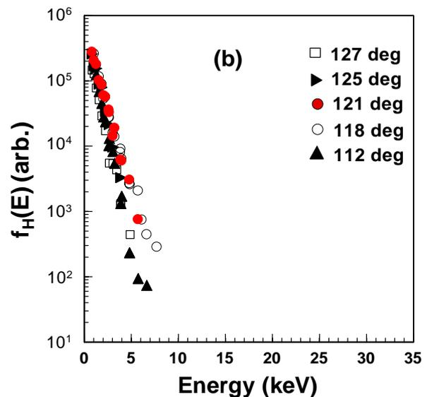
Fig. 4. Minority hydrogen energy spectra for various pitch angles in the high bumpy configuration (a) and in the medium bumpy configuration (b).
