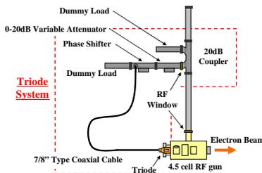
Fig. 4: Schematics of the triode rf gun system.
