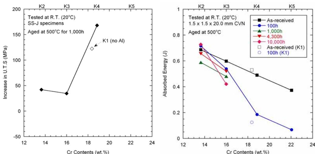
Fig. 1 (left): Cr-dependence of increases in UTS obtained from tensile tests after thermal aging at 500 °C for 1,000 h.
