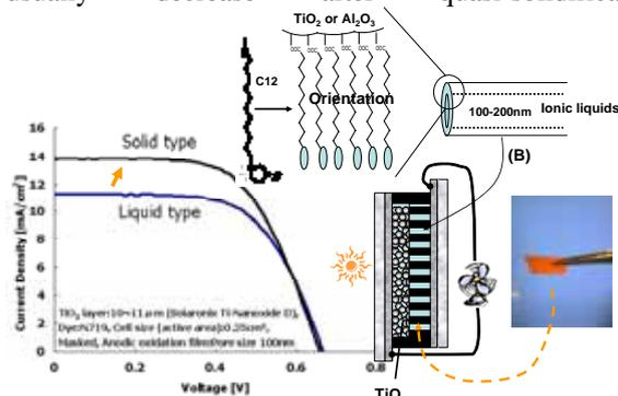
Figure 4 Photovoltaic properties for quasi-solid DSCs consisting of surface modified Al<sub>2</sub>O<sub>3</sub> films
