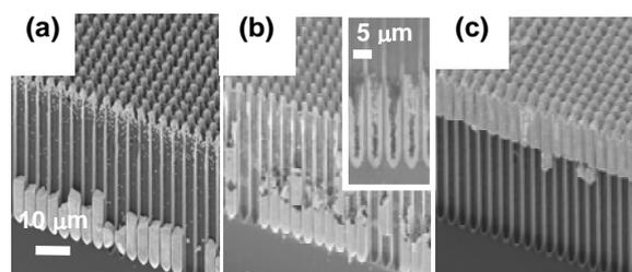
Fig. 5-2 Tilted cross-sectional SEM images of PS electrodeposited for 1 hour: (a) at -0.3 V in 0.1 M  $\text{H}_2\text{PtCl}_6$  + 0.5 M NaCl, (b) at -0.4 V in 0.1 M  $\text{PdCl}_2$  + 0.2 M HCl + 0.5 M NaCl, (c) at 0 V in 0.1 M  $\text{HAuCl}_4$  + 0.5 M NaCl.
