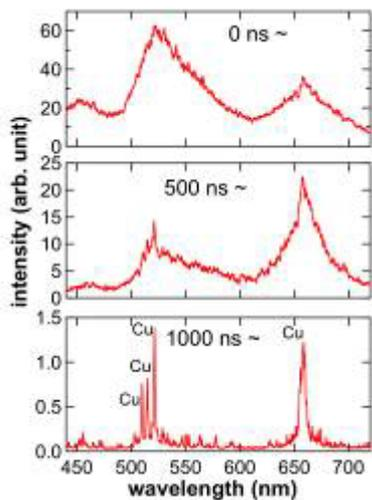
Fig. 2-2. Copper atomic line spectra obtained by the time gate using AOM. The gating time is given in each spectrum.
