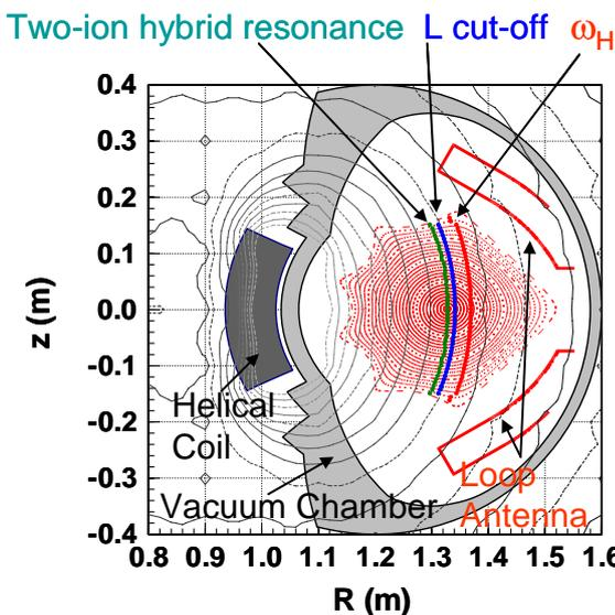
Fig. 3. Two ICRF antennas in the corner section of Heliotron J.
