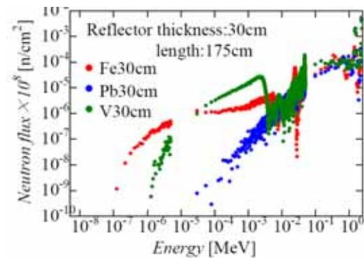
Fig.4(a) Energy spectrum with metal reflectors.
