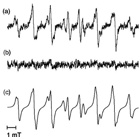
**Figure 3.** EPR spectra obtained for PBS (pH 7.4) containing (a) 4 mM RDEF, 4 mM NADH and 20 mM CYPMPO, (b) 4 mM RDEF, 4 mM NADH, 20 mM CYPMPO and 2,000 units/ml SOD. The reactions were performed for 1 h at room temperature in the dark in an open system and measured by using EPR spectroscopy. (c) Computer-simulated spectrum for the mixture of  $\cdot\text{O}_2^-$  and  $\cdot\text{OH}$  adduct of CYPMPO.
