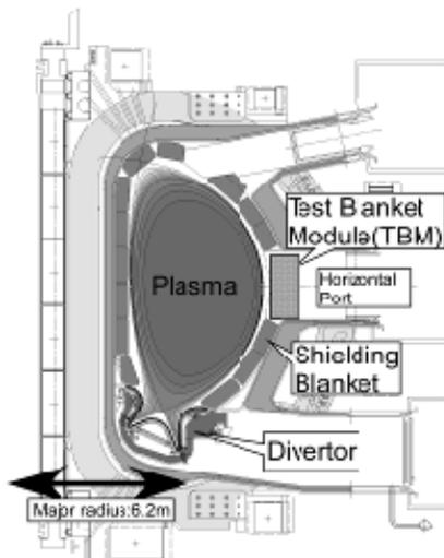
Figure 1 Cross-section of ITER
