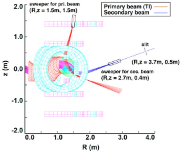
Fig. 2. HIBP system and poloidal cross-section of Heliotron J. Red and blue lines are primary ( $TI^{1+}$ ) and secondary ( $TI^{1+}$ ) beam. There are two sweepers for the spatial measurement.
