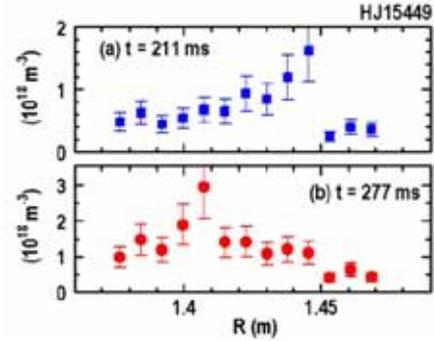
Fig. 7. Density profiles along the divertor probe array at two timings of a single discharge. (The same discharge as in figure 4.)
