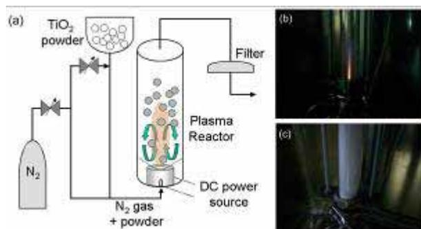
**Fig. 5** Non-equilibrium nitrogen DC-arc plasma apparatus with a vertical type reactor: (a) Schematic illustration, (b) typical nitrogen plasma without powder feeding, and (c) nitrogen plasma treatment with powder feeding. (Y. Suzuki et al., *J. Nanosci. Nanotech.*, in press)
