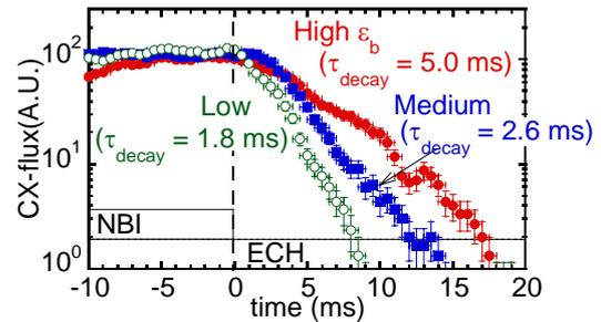
Fig. 4 Time evolution of CX flux ( $E = 18$  keV) after turning-off of NBI. The acceleration voltage of NBI was 28kV and CX-NPA observed the slowing down of beam ions. The base plasma was sustained by 70 GHz ECH.
