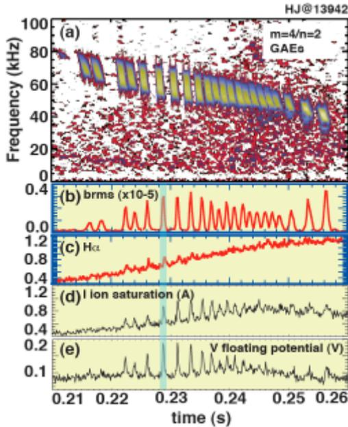
**Fig. 2.** Time evolution of (a) frequency spectrum and (b) amplitude of observed  $m=4/n=2$  GAEs, (c)  $H_\alpha/D_\alpha$  signals, and (d) ion saturation current and floating potential obtained from Langmuir probes.
