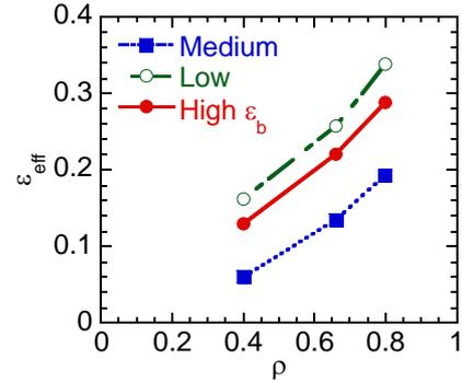
Fig. 1. Radial profile of effective helical ripple deduced by DCOM in high, medium and low  $\varepsilon_b$  configurations.
