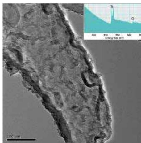
**Fig. 6** TEM micrographs of a unique nanowire-network structure existed in TiO<sub>2</sub> aerogel/TiO<sub>2</sub> nanowire composite: (Insert) EELS spectrum of the composite. (Y. Suzuki et al., *Nano*, in press).
