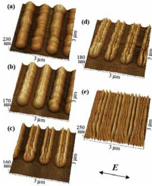
**Fig.5.** SPM images of the DLC stripes irradiated with (a)  $N = 100$ , (b)  $N = 200$ , (c)  $N = 300$ , (d)  $N = 500$  and (e)  $N = 1000$  at  $F = 70 \text{ mJ/cm}^2$ . The arrow denotes the polarization direction.
