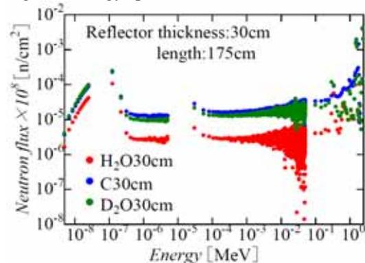
Fig.4 (b) Energy spectrum with light element reflectors.
