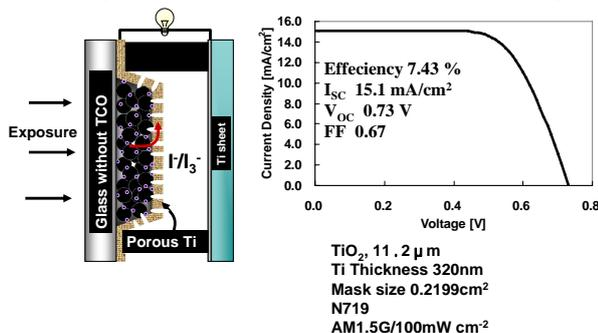
Figure 3. Photovoltaic properties for TCO-less-DSC (all metal electrode)
