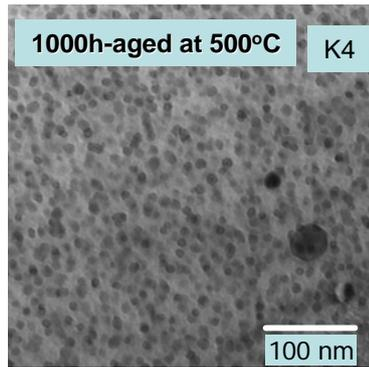
Fig. 3 TEM micrograph of K4 ODS steel after thermal aging at 500°C.
