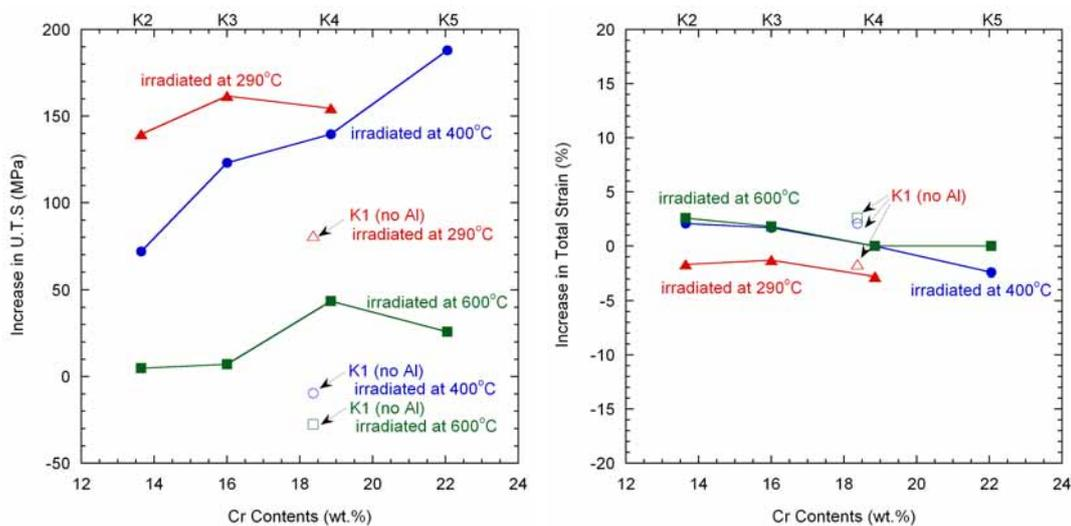
Fig. 4 Tensile test results, a) UTS, b) total elongation, after neutron irradiations at 290, 400 and 600°C.
