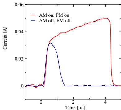
Fig. 8 Wave form of the electron beam injected to the accelerator tube
