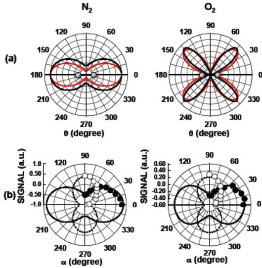
**Fig.3.** The squared asymptotic wavefunction of HOMO of  $N_2$  and  $O_2$  (red) and the angle-dependent HHG signals for a molecule (black), and (b) the measured and calculated  $\alpha$ -dependent signal modulations  $S_1 - S_0$  and  $S_2 - S_0$ .
