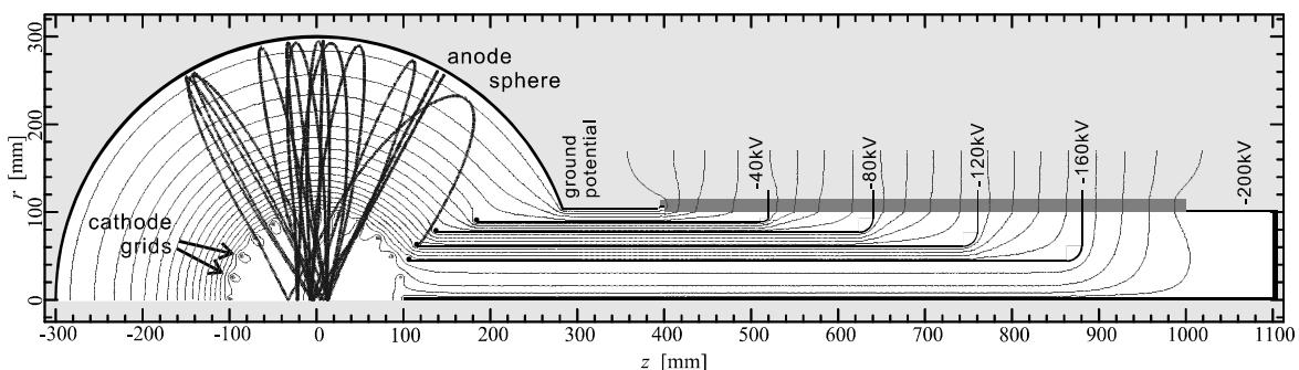
Fig. 4. Cross-sectional view of an IEC with a 5-stage high voltage feedthrough, calculated potential contour lines and ion trajectories
