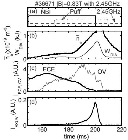
Fig. 1. Typical time evolution of plasma quantities in the NBI plasma startup discharge.
