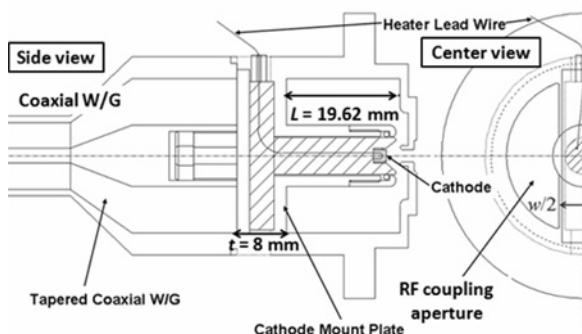
Fig. 3. Cross-sectional views of a prototype coaxial rf cavity for the triode rf gun system
