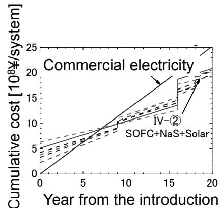
Fig. 5 Cost estimate of the DC microgrid based on the NEDO prediction.
