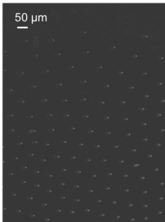
Fig. 3-1 Optical microscope image of polystyrene particles self-assembled at the vertical interface of water and *n*-decane.
