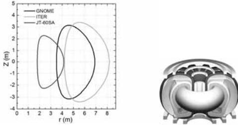
Fig. 2 Comparison of GNOME plasma with ITER and JT-60SA.
