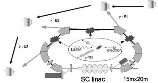
Fig. 4. Conceptual drawing of the ERL Compton- $\gamma$  NRF facility
