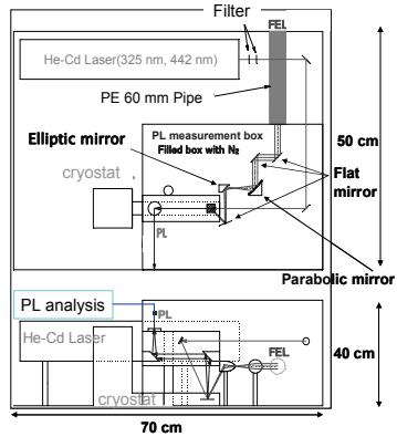
Fig. 2. schematic diagram of MIR-FEL Pump Photoluminescence (PL) Measurement System
