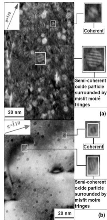
Fig. 1 Weak beam dark field image of the oxide particles dispersed in the matrix of SOC-9 (a) and two-beam dynamical bright field image of the oxide particles dispersed in the matrix of SOC-9-ET-1 (b).
