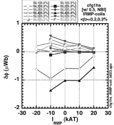
Fig.1.  $m=2/n=1$  magnetic island width as a function of RMP coil current.
