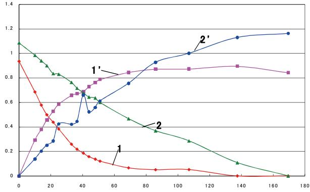
Figure. 1. Time-course (hr) of the intensity after the addition of A3G. Peaks 1 and 2 correspond to each cytosine in the substrate site located close to either 5' or 3' end, respectively. Peaks 1' and 2' correspond to each uracil converted from the two cytosines, respectively.
