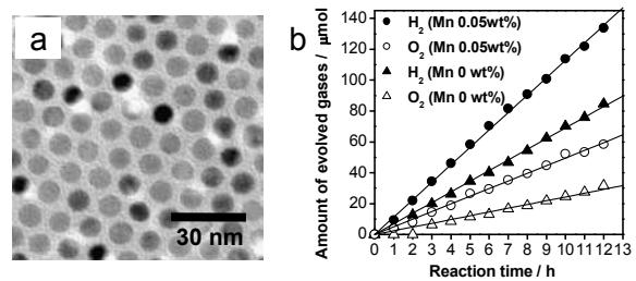
Fig. 2 (a) TEM image of  $9.2 \pm 0.4$  nm MnO NPs and (b) overall water splitting under visible light ( $\lambda > 420$  nm).
