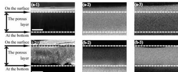
Fig. 2-1 Cross-sections of chemically-modified microporous silicon after platinum electrodeposition observed and analyzed by SEM and EDS. The images of (a-1), (a-2) and (a-3) show an SEM image, EDS mapping of Si and Pt of a microporous silicon substrate modified with propiolic acid. The images (b-1), (b-2) and (b-3) are the same as the upper ones but obtained with a microporous silicon substrate modified with methyl propiolate.
