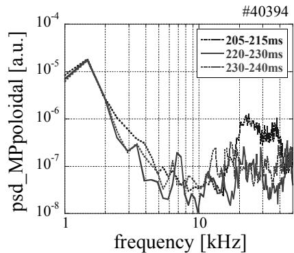
Fig. 4. An example of power spectrum of poloidal magnetic fluctuation for three different timing of a single discharge. The SMB injected at  $t = 218 \text{ ms}$ . A coherent fluctuation are only observed in the 7-8 kHz just after the SMBI ( $t = 220\text{-}230 \text{ ms}$ ).
