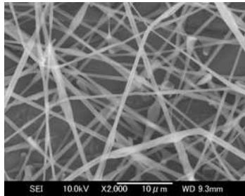
**Fig. 1** SEM image of electrospun P3HT–PVP (1:3) nanofibers.
