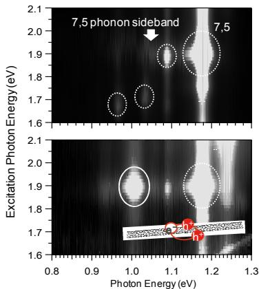
Fig. 1-1 Photoluminescence excitation map hole-doped single-walled carbon nanotubes. Upper panel: without hole-doping of CoMoCAT SWNT, Lower panel: with hole-doping
