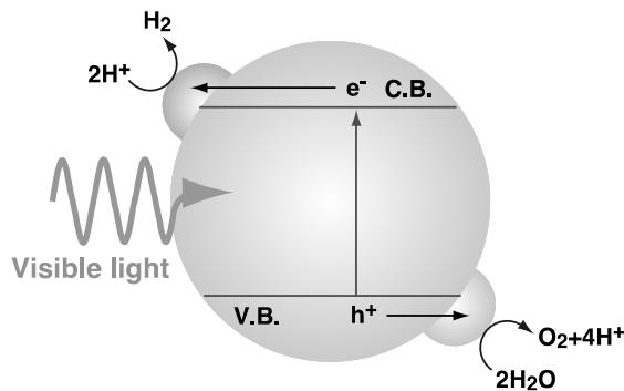
Fig. 1 Schematic of visible light-driven overall water splitting over semiconductor photocatalyst modified with two different cocatalysts.
