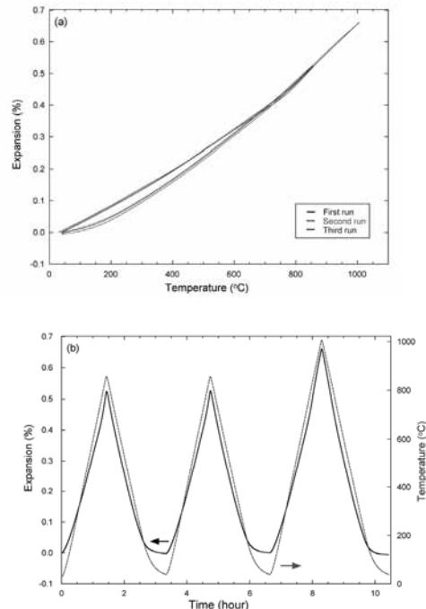
**Fig.3** Bulk thermal expansion of porous MgTi<sub>2</sub>O<sub>5</sub> sintered at 1100°C. Up to 850°C for the first and second runs, and 1000°C for the third run. (a) Thermal expansion curves, and (b) expansion vs. time plot. (Y. Suzuki and M. Morimoto, *J. Ceram. Soc. Jpn.*, **118** (2010)1212)
