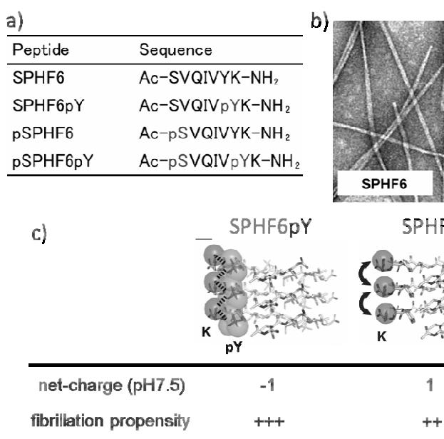
Figure 2 a) PHF6 derivative peptides. Abbreviations: pY, phosphotyrosine; pS, phosphoserine; Ac, acetyl group. b) TEM images of fibrous aggregates of SPHF6 derivative peptides. All samples were transferred directly from reaction mixture to carbon-coated grids and stained with 2% phosphotungstic acid. Scale bar: 100 nm. c)
