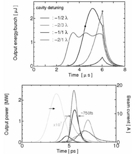
Fig. 3 Macropulse and micropulse time structure in the case of using JAEA undulator when the total cavity loss is 8%.
