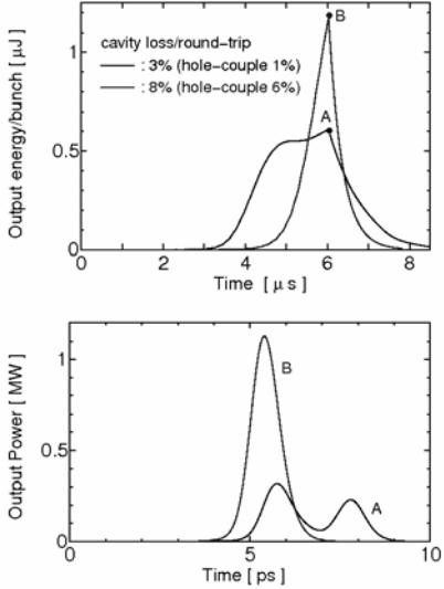
Fig. 1 Macropulse and micropulse time structure depending on the cavity loss when the cavity detuning is  $-l$ .
