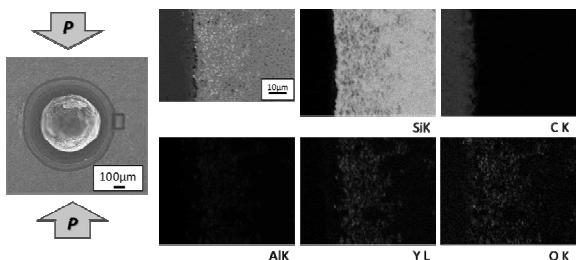
Fig. 2-1, EDS analysis result at SiC matrix/coated particle interface
