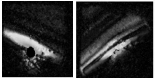
Fig. 3. Example of the phase images of edge plasma fluctuation observed at a plasma section (left: top view, right: side view). Although the scale is not the same, the exposure timing is the same. The filamentary structure elongated to the direction of the magnetic field is observed.
