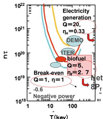
Fig. 1 Schematic illustrations of target of Plasma power balance  $Q$  value for biomass-fusion hybrid GNOME.
