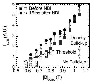
Fig. 2. Comparison of ECE intensity in the case of the successful and unsuccessful density build-up discharges.
