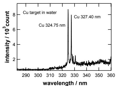
Fig. 5-1 Optical emission spectrum of Cu atoms in the laser plasma produced by the irradiation of Cu target in water by the multi-pulse microchip laser.
