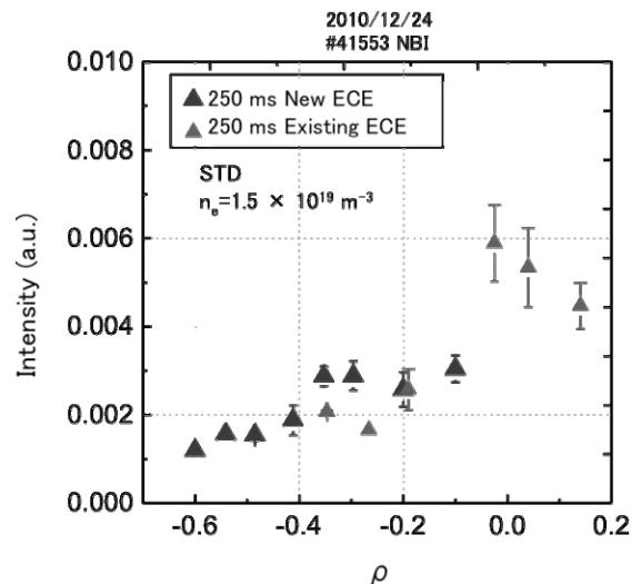
Fig. 1. Electron radiation temperature profile measured with new and existing ECE radiometers.
