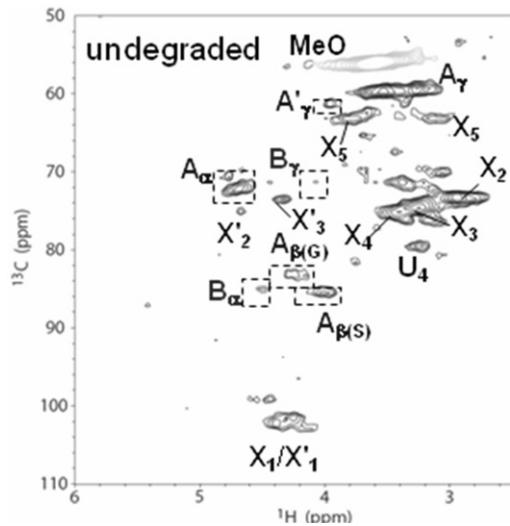
Figure. 3  $^1\text{H}$ - $^{13}\text{C}$  HSQC spectrum of all components of wood biomass. A and B indicate lignin peaks and X and U indicate polysaccharide peaks.
