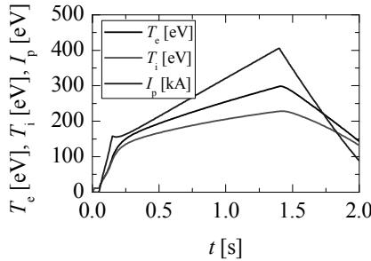
Fig. 2. Temporal behaviors of  $T_e$ ,  $T_i$ , and  $I_p$  on JT-60SA configuration
