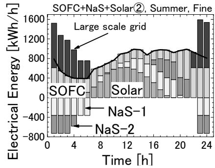
Fig. 4 Operation daily power profile of the DC microgrid on a summer day
