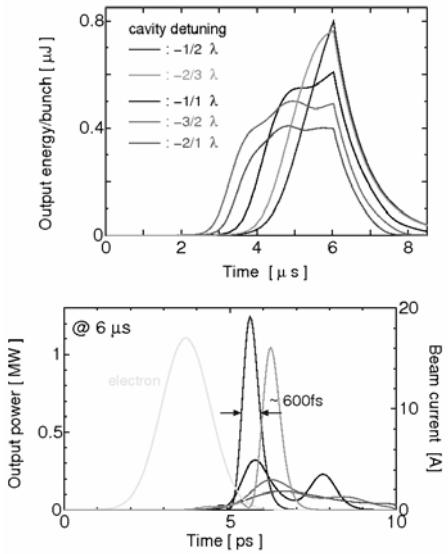
Fig. 2 Macropulse and micropulse time structure depending on the cavity detuning when the total cavity loss is 3%.
