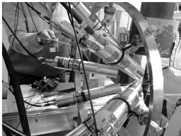
Fig. 4 \text{LaBr}_3(\text{Ce}) scintillator array detector tested at HI \gamma S facility.
