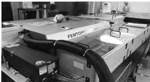
Fig. 1. CEP stabilized Ti:sapphire CPA laser system (5 fs, 0.1 TW, 1 kHz).
