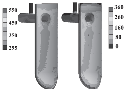
Fig. 2: Example distributions of temperature and stress on the inner RPV wall after 1200s
