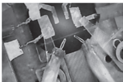
Fig. 2. Photograph of TE measurement for Au-patterned SWNT mat. Outer and inner pairs of electrodes were utilized for current and voltage measurements. Bare probes separated by line drawn by razor blade on the other sides of circular SWNT mat was utilized for temperature measurement.
