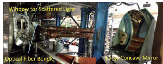
Nd:YAG laser Thomson scattering system installed in Heliotron J
