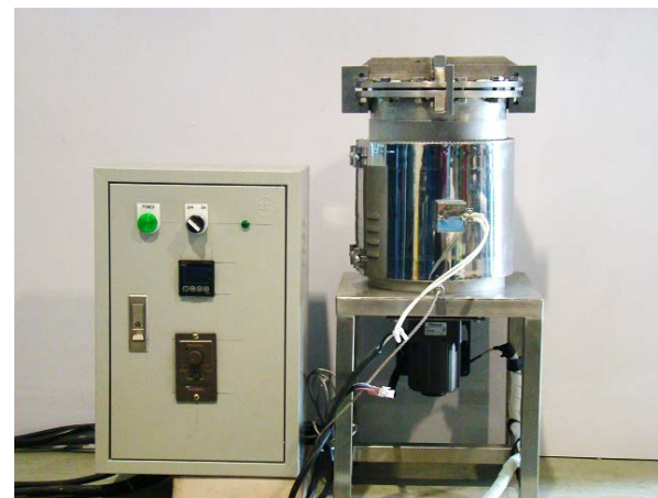
Fig. 2 Autoclave (made in RMUTT) for nanomaterials preparation.
