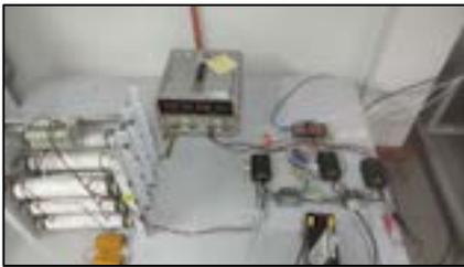
Fig.1. Experimental setup for battery capacity test.
