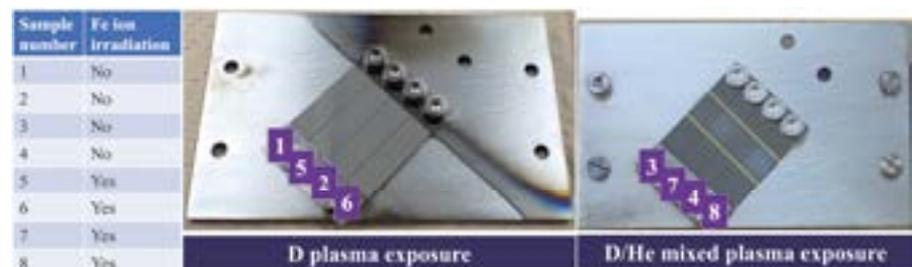
Fig. 1. Sample number as well as pictures after D plasma exposure and D/He plasma exposure experiments.
