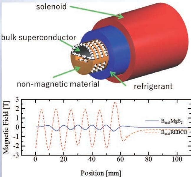
Periodic magnetic field can be generated by applying magnetic field to the stacked array which consists of bulk superconductors and non-magnetic materials. Different superconductor family can generate periodic magnetic field with different features. Red dotted line: strong periodic magnetic field (Rare earth cuprate superconductor, REBCO). Blue line: precise periodic magnetic field (magnesium diboride,  $MgB_2$ )
