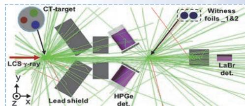
Isotope CT by using Laser-Compton Gamma-ray beam
