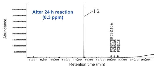
D. The result of reacting 40 mg L<sup>-1</sup> of commercial PCBs with composite type of catalytic enzyme, it degraded to 0.3 mg L<sup>-1</sup> in comparison with the control (top) within 24 hours (bottom). PCBs was analyzed by gas chromatograph quadrupole mass spectrometer.
