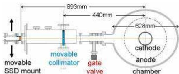
Fig. 2. A cross-sectional layout of spherical anode and cathode grids installed inside a vacuum chamber, a collimator whose aperture is 12 mm $\phi$ , and an SSD set in a linearly movable mount.
