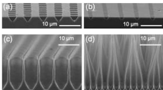
Fig. 2-1 (a) and (b) show the ordered pre-etch patterns with different sizes. (c) A cross-sectional SEM image of an ordered macropore. The etching was preformed using the substrate shown in (a). (d) A cross-sectional SEM image of silicon nano-wires. The nanowires were formed by control of applied current leading to the selective dissolution of the pore walls.
