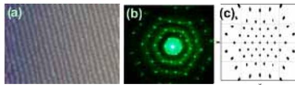
Fig. 5-2 Ordered monolayer of polystyrene microsphere on a glass substrate. (a) optical microscope image, (b) laser diffraction pattern on a plane screen, and (c) simulation of the laser diffraction pattern by projecting the Laue function to x-y plane.
