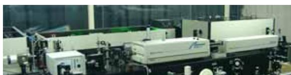
Fig. 1. High-intensity, 40-fs Ti:sapphire laser system.
