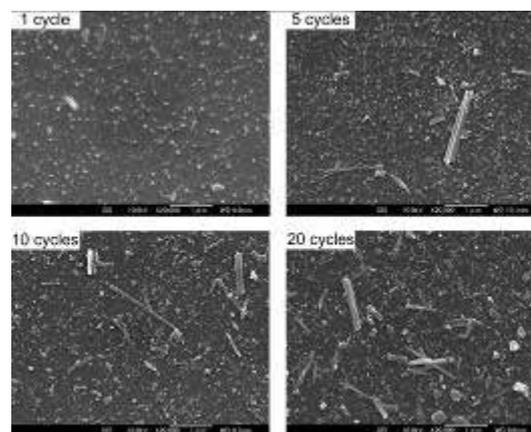
**Fig. 4** Preparation and Microstructure of titanate-nanowire thin films prepared by spray-LbL method (the scale bars are 1 μm). (Y. Suzuki et al., *J. Ceram. Soc. Jpn.*, **2009**, 117(3), 381-384).
