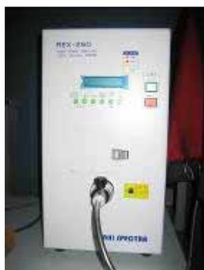
**Figure 2.** REX-250 Mercury Light Source
