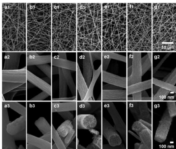
er-by-Layer (spray LbL) method within a short time. Due to the good dispersion state of the nanowires in an aqueous suspension and their linear morphology, titanate nanowires effectively adsorbed on the glass substrate. As a reference, TiO<sub>2</sub>-anatase nanoparticle thin films were also prepared by spray-LbL method. This work was supported by MEXT, Japan (Grant-in-Aid for Science Research No. 19685020 For Young Scientist: Category A).
