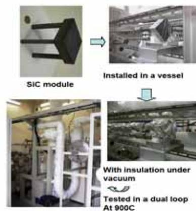
Fig.3. heat exchanger tested in a He-LiPb loop.
