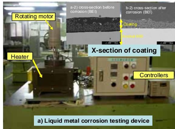
Fig. 3 a) developed liquid corrosion testing device before installing into a glove box, b, c) cross-sectional view of coating before and after LBE corrosion test.
