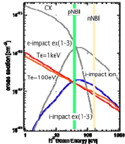
Fig.1 Cross sections of the atomic processes relevant to the BES diagnostics for the Balmer-alpha beam emission.
