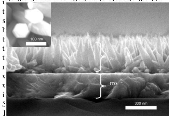
**Fig. 1** SEM cross sectional image of ZnO nanorod arrays on the ITO substrate. Inset shows the top view image (T.S., S.Y. *et. al.*, *Solid-State Electronics*, 2009, 53, 176-180).
