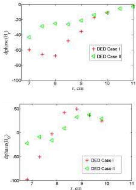
Fig.1. Profiles of phase changes (degrees) of magnetic field  $B_{r,\theta}$  perturbations in HYBTOK-II [6]. These changes are the result of a plasma response.
