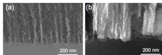
Fig. 3-1 Cross-sectional SEM images of mesoporous silicon (a) and that after filling with copper by electrodeposition (b).
