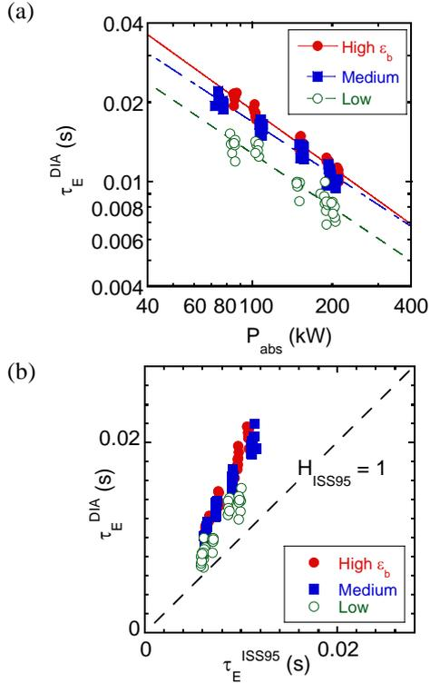
Fig. 2 Experimentally obtained energy confinement time as a function of (a) NBI absorption power, and (b) International Stellarator Scaling law ISS95.
