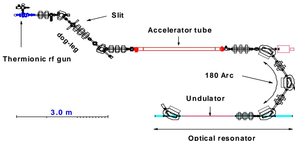
Figure 1: Layout of KU-FEL system
