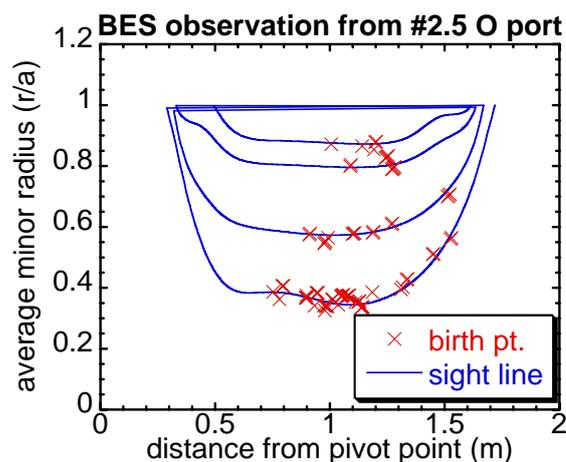
Fig.3 Location of the birth points and the sight lines in Fig. 2 represented in the average minor radius. The horizontal axis is the distance from the datum point for the viewing chords near the observation port #2.5O.
