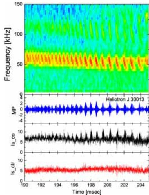
Fig. 3 The contour map of the power spectrum by magnetic fluctuation and filtered waveform, co- and counter-directed ion currents ( $I_{s\_co}$  and  $I_{s\_ctr}$ ) measured by HDLP at  $r/a=0.9$ .
