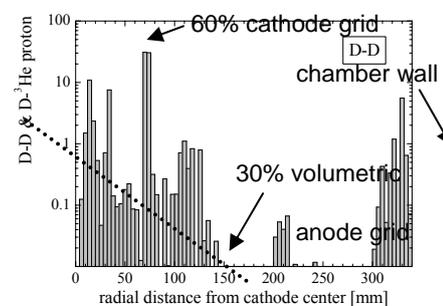
Fig. 3. Reconstructed distributions of D-<sup>3</sup>He and D-D proton yields (fractions in 4-mm thick spherical hulls), with  $V = -60$  kV,  $I = 30$  mA and  $P_{3\text{He}} / P_{\text{D}_2} = 2.3$ .
