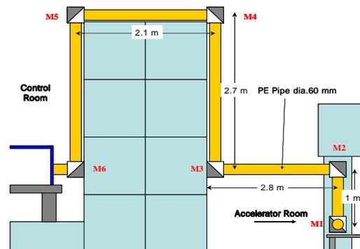
Fig. 4. A schematic drawing of the FEL beam transport. The FEL output is transported from the accelerator room to the control room using flat mirrors and nitrogen displaceable piles.
