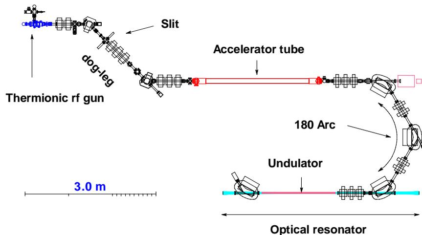
Fig. 1 Schematic drawing of the KU-FEL
