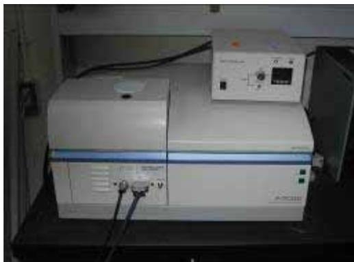
**Figure 1.** F-7000 Fluorescence Spectrophotometer
