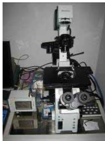
**Figure 3.** IX-81 Mortorized Inverted System Microscope equipped with ImagEM (EM-CCD Camera)
