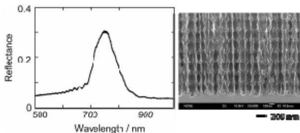
Fig. 4-1 Reflectance spectrum of a medium-sized porous rugate filter prepared by anodization of heavily doped silicon, and the SEM cross-sectional image.
