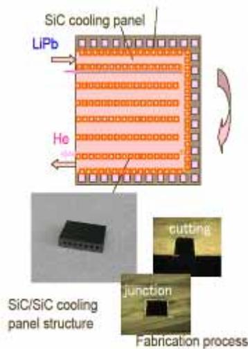
Fig.2. Concept of the high temperature SiC-LiPb blanket.
