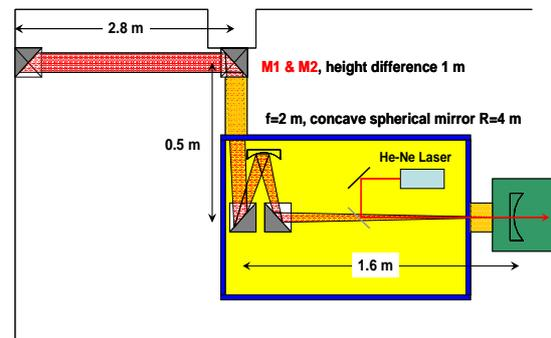
Fig. 3. Schematic drawing of the beam expander consisting of a concave spherical mirror and two flat mirrors.
