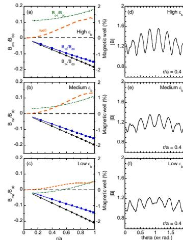
Fig. 1. (a)-(c) Radial profile of magnetic well, helicity, toroidicity and bumpiness in Boozer coordinate systems and (d)-(f) field strength along the field line in the three  $\varepsilon_b$  configurations.
