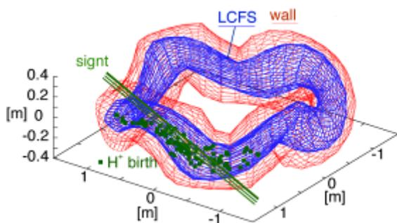
Fig.2 Schematic views of the Heliotron J magnetic flux surface and chamber wall. Birth points of the beam ions (reduced for the visibility) and the possible viewing chords when one intends to keep spatial resolution of the BES system are drawn.
