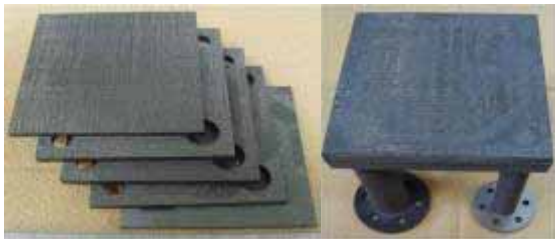
Fig.1 The scale model with 10cm square for compact intermediate heat exchanger (IHX) using the NITE-SiC/SiC composites with channel.
