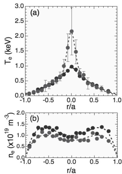
Fig. 1 Typical electron temperature (a) and density (b) profiles with and without the eITB. The plasma density is slightly different in both plasmas. The profiles are measured with Nd:YAG Thomson scattering system.
