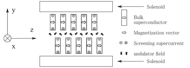
Fig. 4 Conceptual drawing of the bulk HTSC SAU and generation principle of the periodic undulator field using an induced current.
