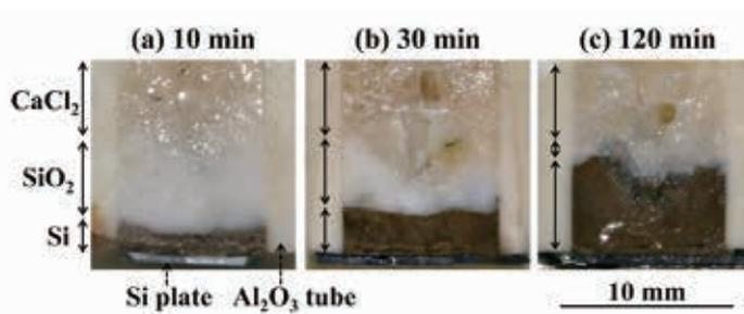
Fig. 1. Cross-section of the working electrode after electrolysis for 10, 30 and 120 min.
