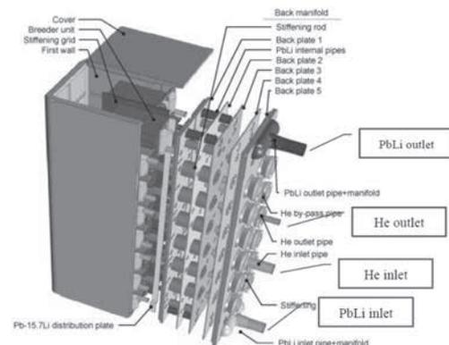
Fig. 1. (a) A schematic of the European HCLL TBM
