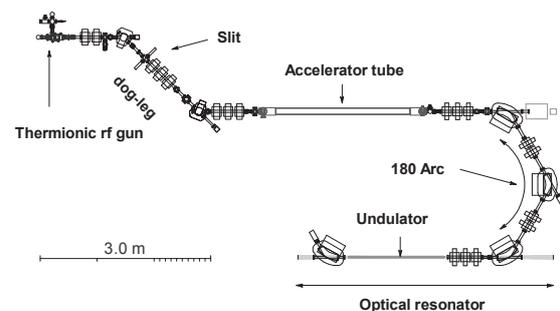
Fig. 1 Schematic drawing of the KU-FEL
