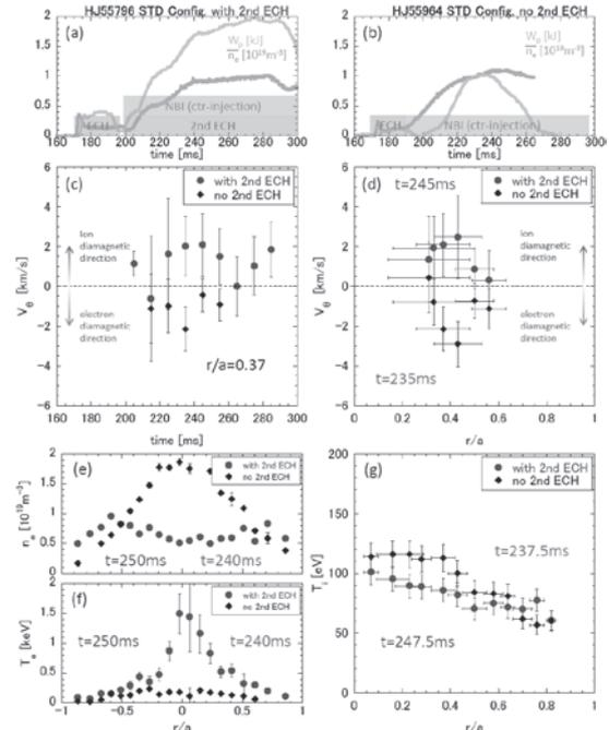
Fig. 3 (a) and (b); time evolutions of  $\bar{n}_e$  and  $W_p$  in the case of with and without 2<sup>nd</sup> ECH plasmas. (c) and (d); time evolution and radial profile of  $v_\theta$ , (e) and (f); radial profiles of electron density and temperature and (g) radial profile of ion temperature in the case of with and without 2<sup>nd</sup> ECH plasmas.
