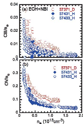
Fig. 3, Plot of (a)  $CIII/n_e$  and (b)  $OV/n_e$  as a function of  $n_e$  with relation to H and D plasmas.
