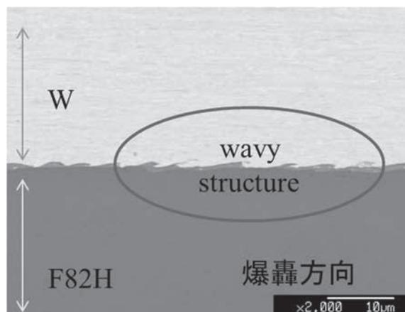
Fig. 2 Cross-sectional SEM image of the interface of W-coated F82H fabricated by underwater explosive welding.
