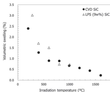
Figure 2: Irradiation effect on swelling of CVD- and LPS-SiC.
