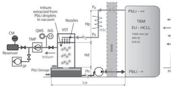
Fig. 2. Vacuum Sieve Tray for HCLL TBM
