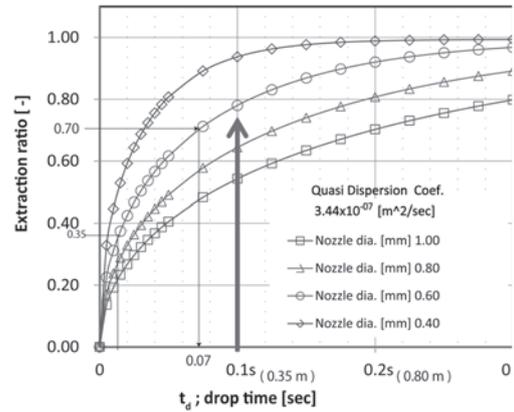
Fig. 3. Estimated extraction efficiency as the function of nozzle size for droplet formation.
