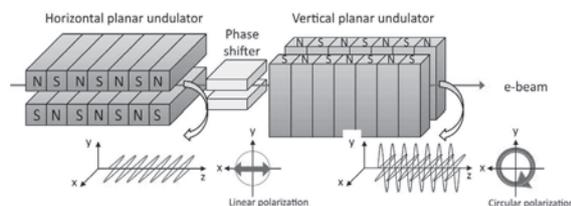
Fig.3: Proposed crossed-undulator configuration for variable polarized THz superradiant. Phase shifter delays the radiation so as to choose proper phase between two undulator radiations.
