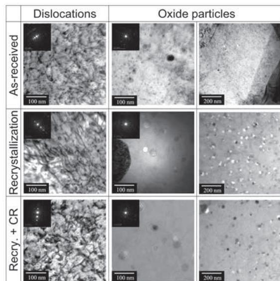
Fig. 1: Dispersion of oxide particles in ODS steel
