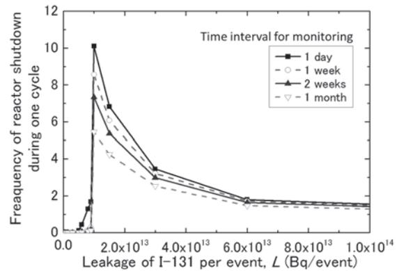
Fig. 2: Frequency of immediate reactor shutdown for a fixed value of the leak rate, when the time interval of intermittent monitoring is changed
