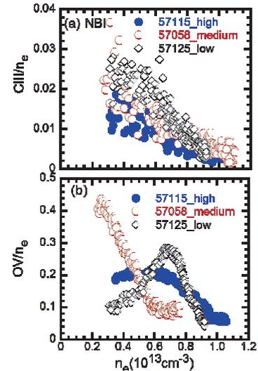
Fig. 1, Plot of (a) CIII/ $n_e$  and (b) OV/ $n_e$  as a function of  $n_e$  with different magnetic configurations.
