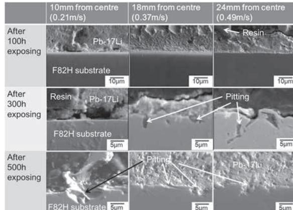
Fig. 1 Cross-sectional SEM images of F82H after immersing in Pb-Li at 600C for 100, 300, and 500 hrs.
