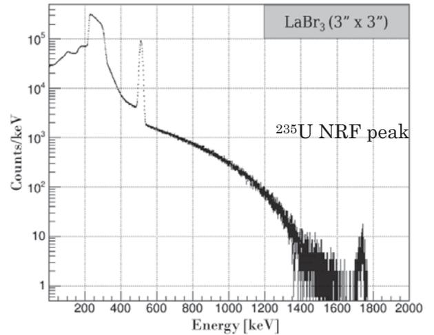
Fig. 5 Simulated energy spectrum from the 3''x3'' LaBr<sub>3</sub>(Ce) scintillator array detector.
