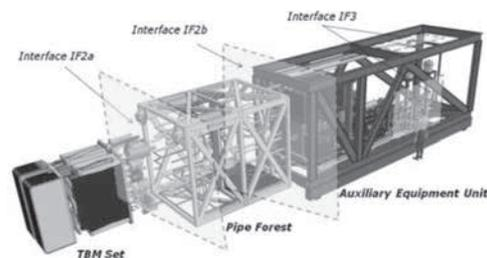
Fig. 1. (b) TBM system for HCLL.
