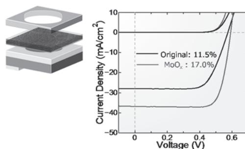
Figure 1: Photovoltaic performance of carbon nanotube solar cells using metal oxide layers.
