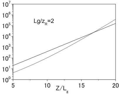
Fig.2. The diffraction effect on exponential gain for different ratio of gain length and Rayleigh length. The red line: our numerical result; The black line: the result from the diffraction correction on the gain length by Xie Ming's experience formula.
