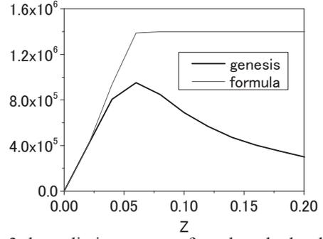
Fig.3 the radiation power of pre-bunched e- beam,  $l_b \approx 4\lambda_s$ ,  $b_0=0.86$ . The red line: the result of the formula (3); The black line: the result of Genesis simulation.
