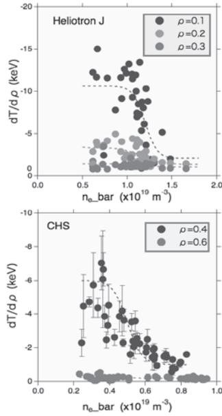
Fig. 2 Density dependence on the temperature gradient in the core region and the outside of the steep temperature gradient for Heliotron J and CHS plasmas.
