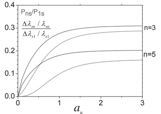
Fig.4, Gain length, the saturation power and the bandwidth of the liner harmonic with the undulator parameter.
