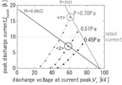
Fig.2 I-V curves of glow discharge at different gas condition.
