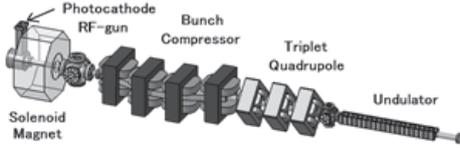
Fig. 3 Schematic view of the compact seeded THz-FEL amplifier.
