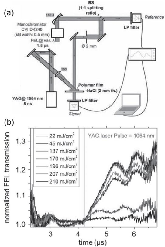
Fig. 3 (a) Experimental setup. (b) Temporal change of transmission of the FEL pulse at 13.7  $\mu\text{m}$  as a function of YAG laser fluence.
