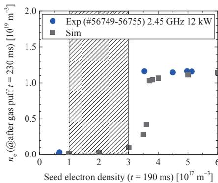
Fig. 1 Dependence of electron density after gas puff on seed electron density.
