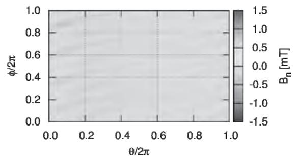
Fig.3: The normal field component on the first wall of the vacuum vessel.
