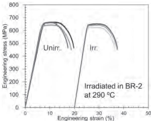
Fig.2 Engineering stress–strain curves of cryo-rolled CuCrZr alloy before and after neutron irradiation in BR2 at 290 °C.
