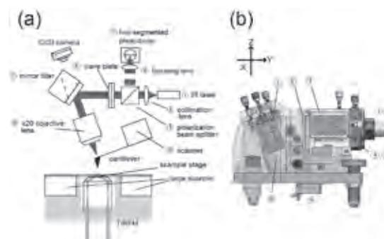
Fig. 2 Schematics and photograph showing the tip-scan HS-AFM unit. (a) Configuration of OBD detector with dichroic mirror tilter. (b) Whole structure of the tip-scan HS-AFM unit. The numbers attached to respective parts correspond to the numbers shown in (a). (c) A photograph of the tip-scan HS-AFM unit mounted on the optical stage in which the wide-area XY-scanner is installed.
