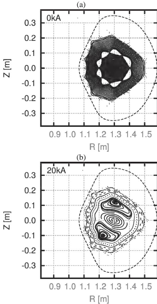
Fig.2: Poincaré plots of magnetic field lines with and without the RMP are shown at a poloidal cross section of  $\phi = 0$ .
