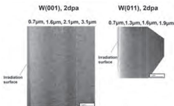
Fig. 1: Microstructure of 2 dpa irradiated W{001} and W{011}. The position of deeper ion-irradiation affected zone is much deeper in W{001}.
