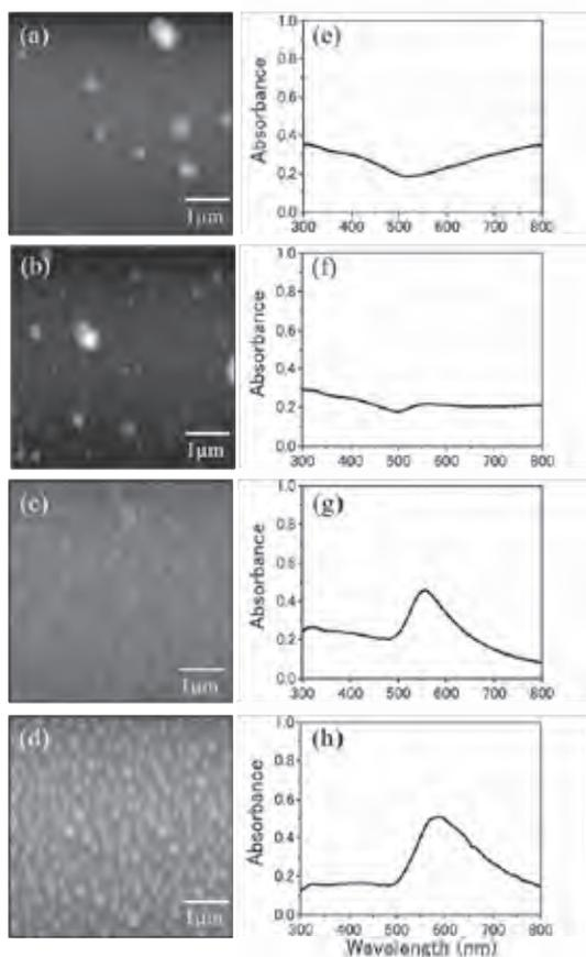
Fig. 3 AFM images (left column) and optical absorption spectra (right column) of 5 nm Au films on cover glasses after CO<sub>2</sub> laser annealing at different laser powers. The employed laser powers are (a, e) 0, (b, f) 2.5, (c, g) 4, and (d, h) 6 W, respectively. Irradiation time is 5 minutes for all cases.
