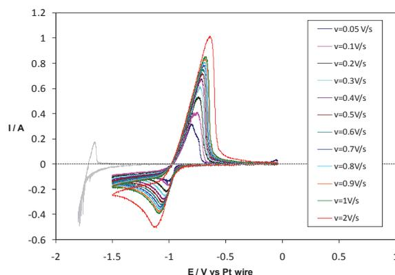
Figure 2. Cyclic voltammetry on Ag in molten KF-LiF-K<sub>2</sub>SiF<sub>6</sub> at  $800^\circ\text{C}$  [7].
