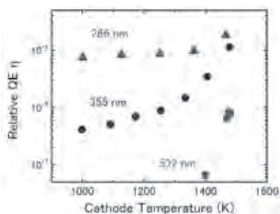
Fig. 1 Temperature dependence of relative quantum efficiency (measured electrons / incident photons) of LaB<sub>6</sub>
