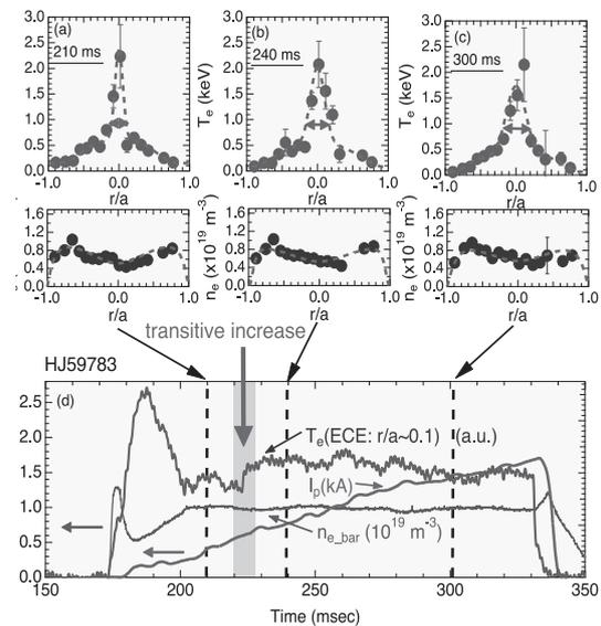
**Fig.1** Rapid electron temperature rise has been observed during eITB formation with current ramp-up. (a) (b) (c) Electron temperature and density profiles. (d) Time evolution of electron temperature, density and plasma current.
