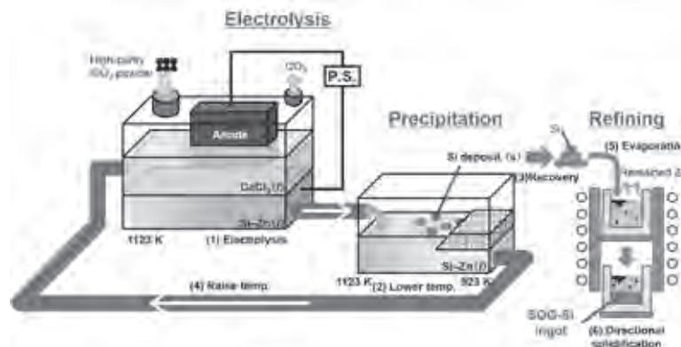
Fig. 1. A schematic drawing of solar-grade Si production utilizing an electrochemical reduction of  $\text{SiO}_2$  powder on a liquid Si-Zn alloy cathode in molten  $\text{CaCl}_2$ .
