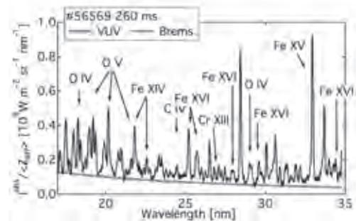
Fig. 1 Calibrated VUV spectrum for high density experiment (#56569) in Heliotron J, for unknown  $\langle Z_{eff} \rangle$ .
