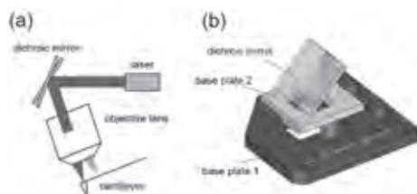
Fig. 1 Dichroic mirror tilter for laser-beam tracking. (a) Schematic showing the working principle of laser-beam tracking by mirror-tilting method. (b) Perspective view of the two-dimensional mirror tilter.
