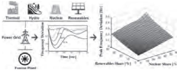
Fig. 1. Peak frequency deviation under the effect of renewable and nuclear power sources.
