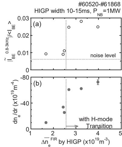
Fig. 4 (a) Root-mean-square of low- $f$  fluctuation and (b) density gradient at peripheral region as a function of density increase by HIGP.
