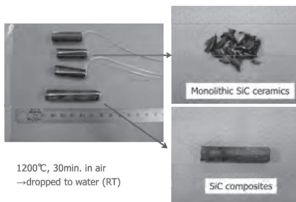
Fig. 3 Monolithic SiC ceramic tubes and BN particle dispersion SiC composite tube before and after thermal shock tests from 1200 °C to ambient temperature.
