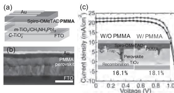
Fig. 2 (a) Schematic of device structure. (b) Cross-sectional SEM image of the device. (c) Photovoltaic performance of perovskite solar cell with and without PMMA layer. Inset shows carrier recombination dynamics.
