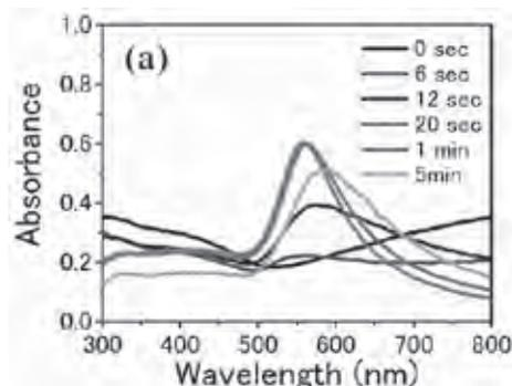
Fig. 4 Absorption spectra of 5nm Au films after CO<sub>2</sub> laser annealing with different irradiation times. Annealing times are (b) 6, (c) 12, and (d) 20 sec, and (e) 1 and (f) 5 minutes, respectively, and the laser power is 6 W for all cases.
