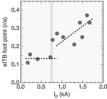
Fig.2 Foot point of eITB as a function of plasma current. Transition occurs at  $\sim 0.7$  kA.
