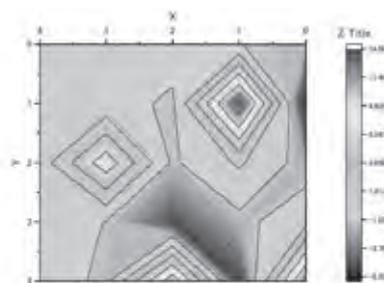
Fig. 3  $^{208}\text{Pb}$  distribution image reconstructed by the transmission of 5292-keV NRF peaks after the normalization.
