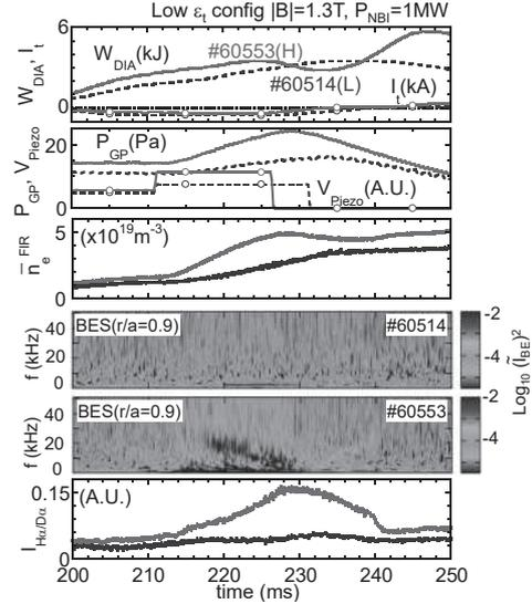
Fig. 3 Time evolution of plasma parameters obtained in H-mode transition (#60553) and no-transition (#60514) plasmas. For the H-mode plasmas, the transition occurs at  $t=240$ ms.
