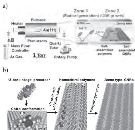
Fig. 1 Schematic illustrations of a) 2Z-CVD instrument and b) synthesis of acene-type GNRs from the Z-bar linkage precursor.
