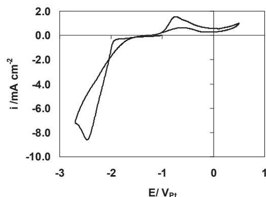
Figure 1. Cyclic voltammetry on Al in [BMP]Tf<sub>2</sub>N saturated with SiCl<sub>4</sub> (~1 M) [5]. Potential scan rate: 10 mV s<sup>-1</sup>
