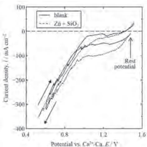
Fig. 2. Cyclic voltammograms for liquid Zn electrodes in molten CaCl<sub>2</sub> at 1123 K. Scan rate: 0.2 V s<sup>-1</sup>.
