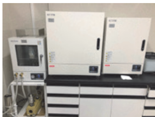
Fig. 1-3 A vacuum oven and box-type dryers.
