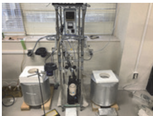
Fig. 1-2 Electric furnaces for molten salt electrolysis.
