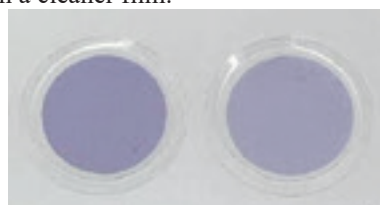
Fig. 5 (6,5) SWCNT film with different thickness
