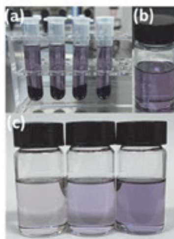
Fig. 1 (a) Solution after centrifugation (the supernatant consists of 65 tubes and the black sediment is impurities). (b) Extracted supernatant (c) Different concentrations of (6,5) solutions obtained by changing the tip sonication time
