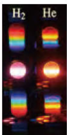
Plasma emits various line spectra as can be seen through a simple grating film. One can draw huge amount of information from the high-grade spectrographs.
