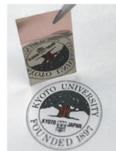
Fig. 1 A photograph of mirror aluminum plating.
